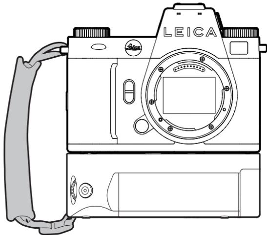
When using the handgrip for portrait photography for extended periods of time, we recommend attaching the carry strap on the strap lug of the camera on the right-hand side and on the strap lug of the handgrip. This will always maintain the camera in the correct position. See p. 36 for instructions on how to attach the carry strap.
