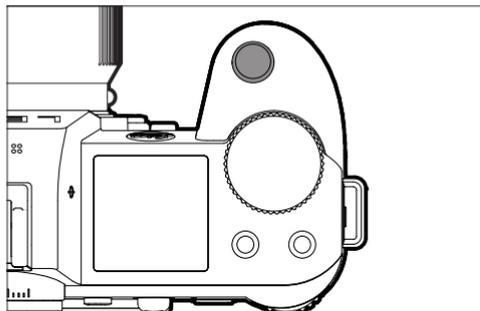
The shutter button works in two stages.
