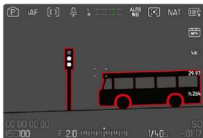
When Focus Peaking is activated,
