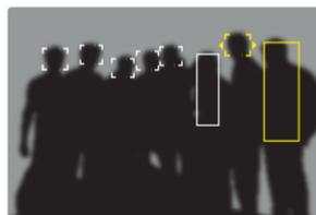
When face detection detects an eye, the focus will be on that eye. Should more than one eye be detected, then the user can choose the eye to focus on. The currently selected eye will be highlighted. Additionally, the desired face can be easily selected if there are several faces in the frame.
