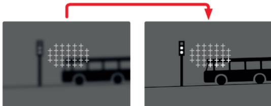
Once the setting has been made, the focus frames are displayed where object sections are displayed in focus.
