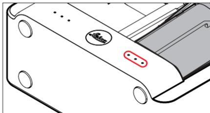
The status LED indicates a correct charging process.
