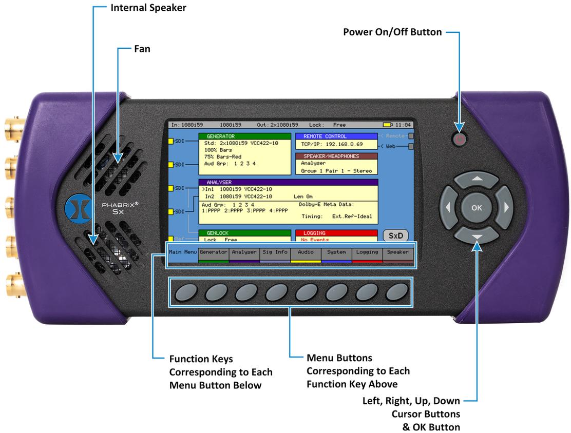
The front panel provides access to the TFT Display and menu system.
