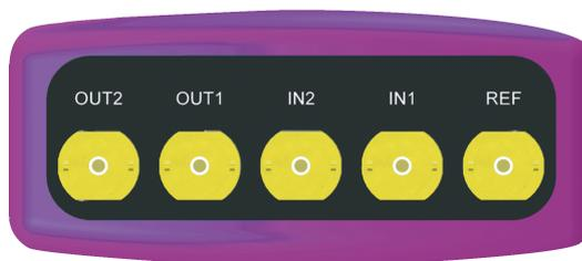
The Sx instrument BNC panel provides the following connections:
