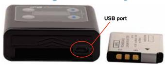
An attached sliding door makes battery installation easy. The USB port is located in the battery compartment.
