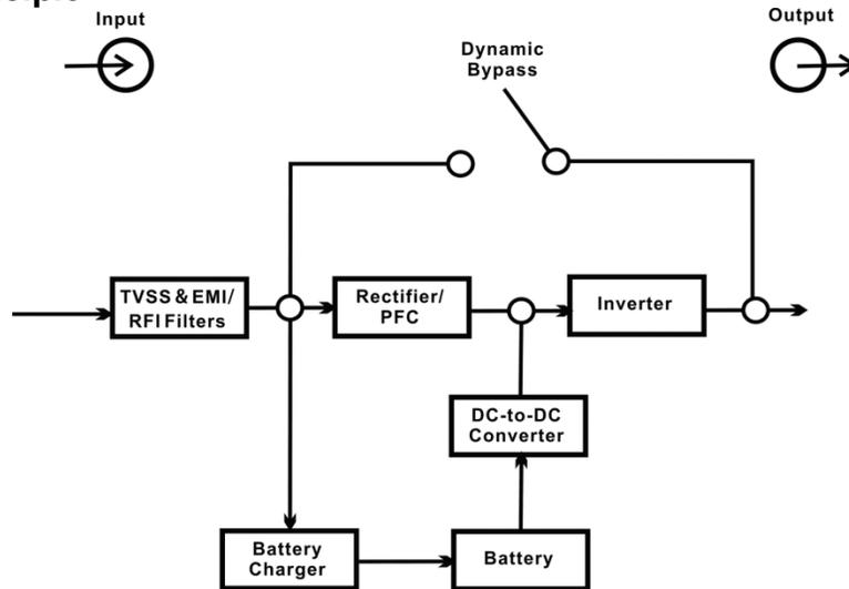
The UPS is composed of mains input, TVSS and EMI/RFI filters, rectifier/PFC, inverter, battery charger, DC-to-DC converter, battery, dynamic bypass and UPS output.
