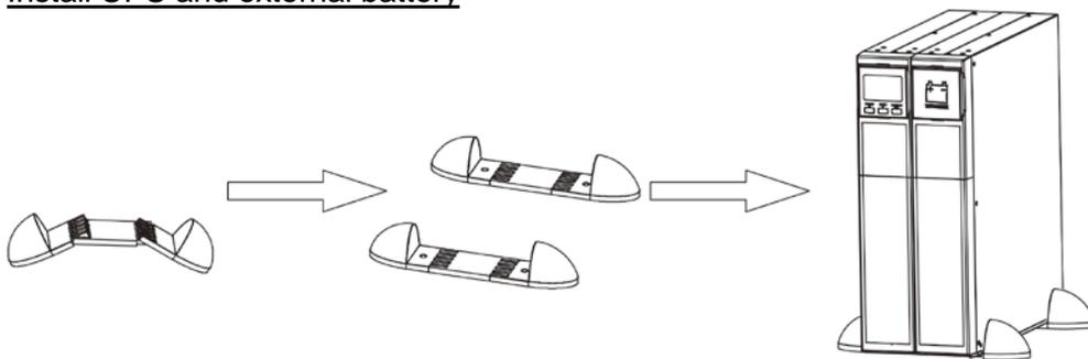
**NOTE:** When installing the UPS or battery pack with feet, keep 2.76in distance from the edge of the unit.
