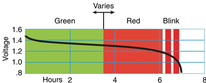
A weak battery will sometimes cause the PWR LED to glow green immediately after the transmitter is turned on, but will soon discharge to the point where the LED will turn red or the unit will turn off completely.
