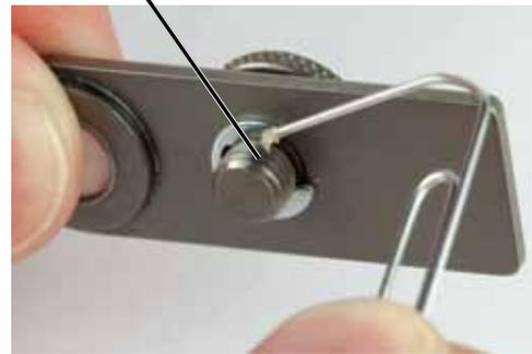
It is not necessary to spread the paste more than a little bit on the thread as the paste will spread itself every time the thumbscrew is screwed in and out of the case during battery changes.
