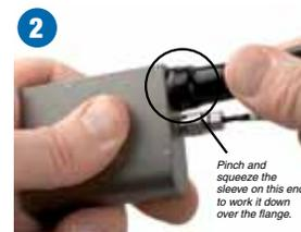
Pinch and squeeze the sleeve near the flange and work it down with a kneading motion over the flange all the way around until it stays in place flush with the housing. Pull on the connector to make sure it is firmly latched.
