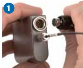
If the sleeve is pulled down and covering the connector, squeeze the end of the sleeve so you can feel the connector inside and press it into the jack until it latches.
