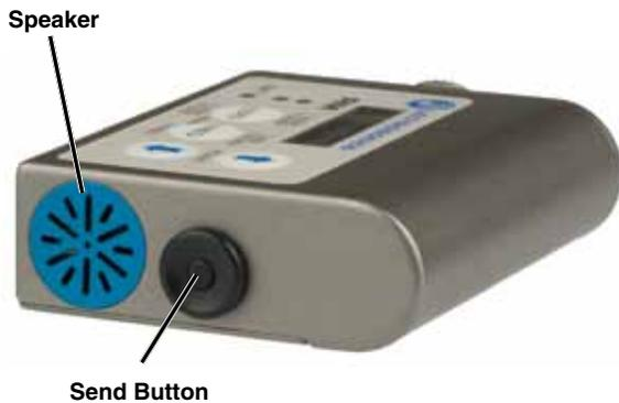
When the transmitter is in the power saving sleep mode, it uses only 20% of the normal battery drain, so battery life will be 5 times longer. This is especially useful in situations where the transmitter is buried deep inside costuming and there are waiting periods between use. The transmitter can “sleep” for several hours and then be awakened and adjusted when the production is about to begin. While the transmitter is asleep, the power LED will blink green every few seconds.
