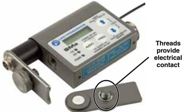
The small enclosed vial contains a tiny amount (25 mg) of silver conductive paste. A small speck of this paste will improve the conductivity between the battery cover plate thumbscrew and the case of the SM.
