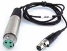
MC41 mic level adapter cable. Female XLR to female TA5F; 37 inches long. Feeds mic level signal to pin 3 on the TA5M jack.
