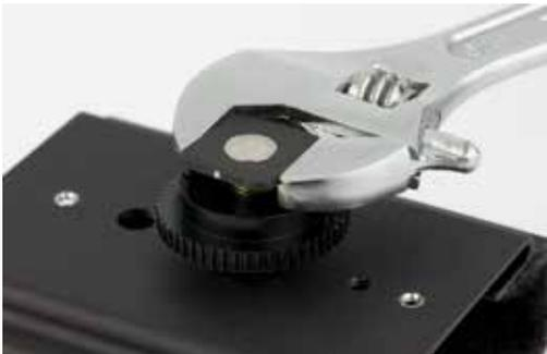
Use a wrench to thread the stud in about 1 - 2 turns, then rotate it to orient the receiver control panel in the desired direction.
