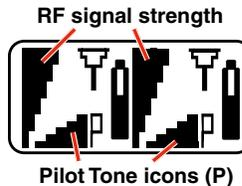
Press the BACK button several times to return to the Main Screen and verify that both transmitters show a strong RF signal strength and that the Pilot Tone icons are NOT blinking (when Pilot Tone is enabled).
