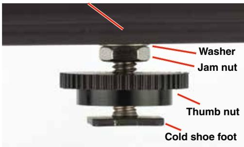
For horizontal mounting, insert the cold shoe foot into the clinch nut in the sleeve. Rotate the foot to the desired position, then tighten the jam nut to lock it in place.
