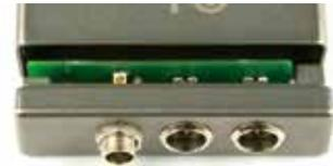
Align the mating connectors and slide the panel straight into the housing until the screw holes align with the housing.
