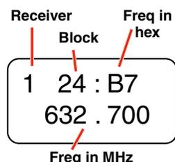
Press MENU/SEL from the Main Window once for Receiver 1 and twice for Receiver 2. The selected receiver is shown in the upper left corner of the LCD.
