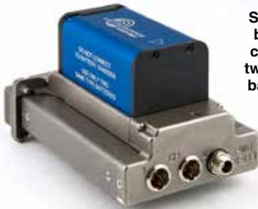
The battery sled adapters do not include charging circuitry. Batteries must be charged with their respective chargers. The adapters include an integral circuit that automatically selects between the battery and the external source, whichever delivers the highest voltage.
