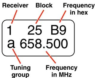
When any tuning mode other than NOR is selected, the frequency screen will include the selected tuning group number.
