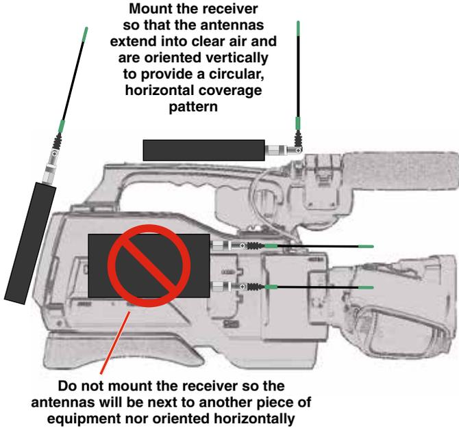
Do not mount the receiver so the antennas will be next to another piece of equipment nor oriented horizontally
