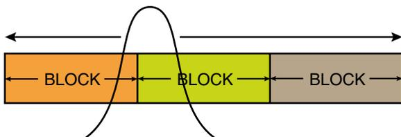
In the front-end circuitry, a tuned filter is followed by an amplifier and then another filter to provide the selectivity needed to suppress interference. This unique filter design allows a wide tuning range and retains the sensitivity needed for extended operating range.
