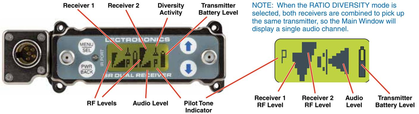
NOTE: When the RATIO DIVERSITY mode is selected, both receivers are combined to pick up the same transmitter, so the Main Window will display a single audio channel.
