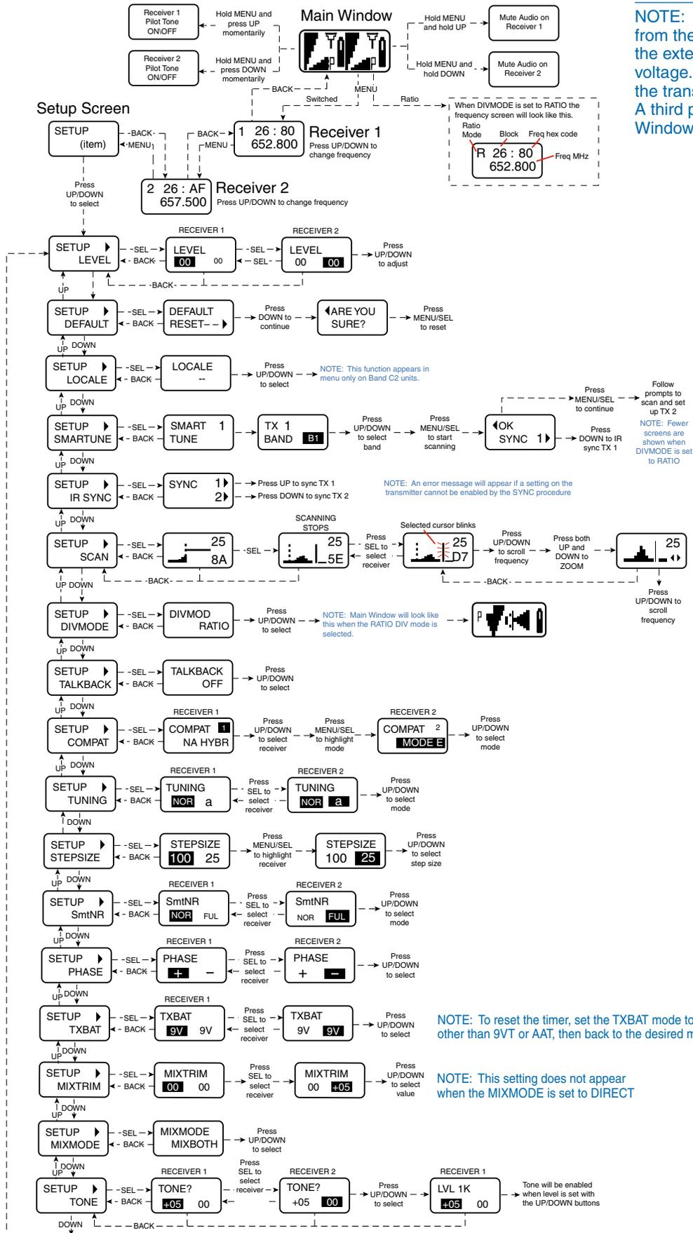
**NOTE:** Press the BACK button from the Main Window to display the external power supply voltage. Press it again to display the transmitter battery voltages. A third press returns to the Main Window.
