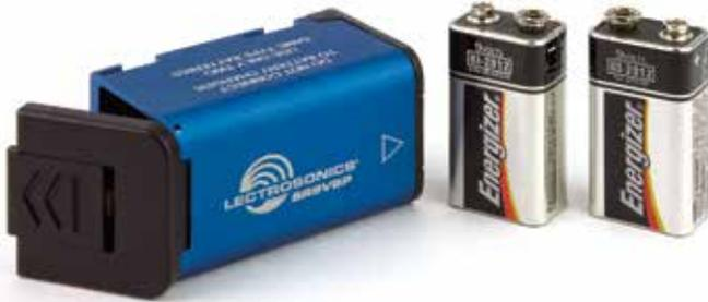
Slide the latch plate in the center of the door outward and swing the door open for access to two 9 volt battery compartments. Polarity barriers in each battery compartment protect against inserting the battery backwards. The circuitry is also protected electrically.
