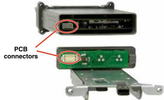
Slide the battery sled adapter into the end of the SR and gently seat it into place with the rear panel flush with the housing.
