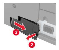
**4** If the printer has a filter cover, then remove the cover.
