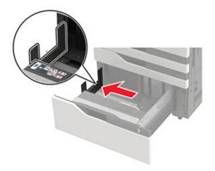
**2** Flex, fan, and align the paper edges before loading.
