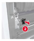
Loosen the screws that secure the transfer belt.
