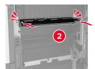
**9** Using the printhead wiper, clean the printhead lens.
