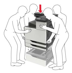
**16** Align the 3000-sheet tray with the printer, and then attach the mounting post.
