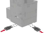
**22** Connect the 2 x 500- or 2500-sheet tray connector to the printer.
