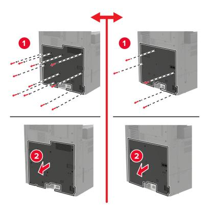
Remove the controller board shield.
