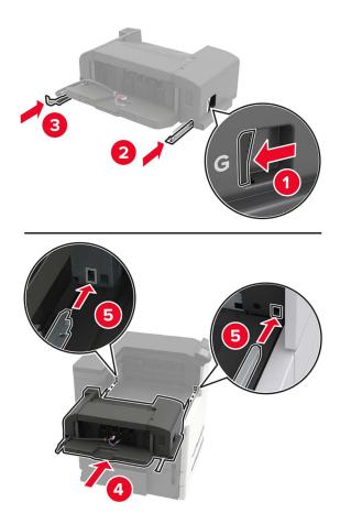
**10** Secure the finisher to the printer.
