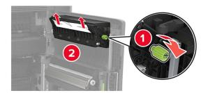
**3** Open the standard trays, and then remove the jammed paper.
