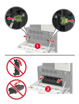
**3** Remove the photoconductor unit.
