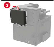
**5** Remove the controller board access cover.
