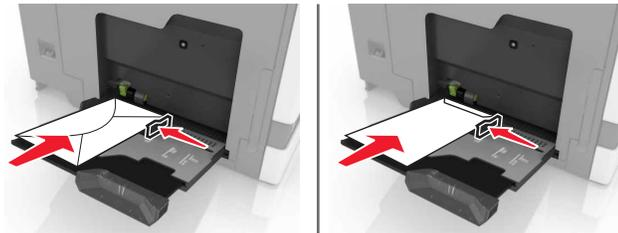
**Warning—Potential Damage:** Do not use envelopes with stamps, clasps, snaps, windows, coated linings, or self-stick adhesives.
