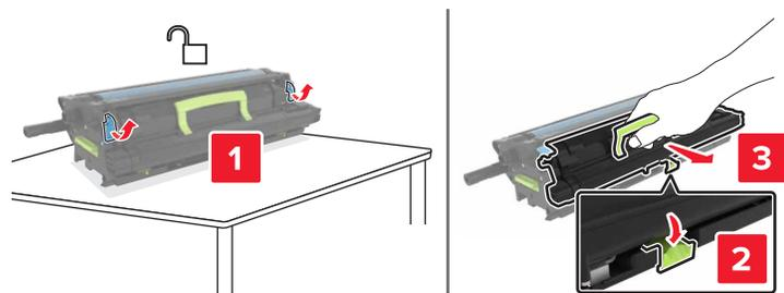
5 Unpack the new photoconductor unit, and then remove the packing material.
