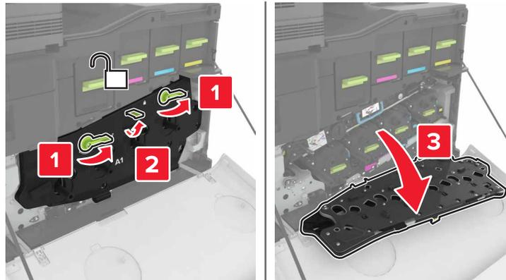
**5** Remove the transfer belt.
