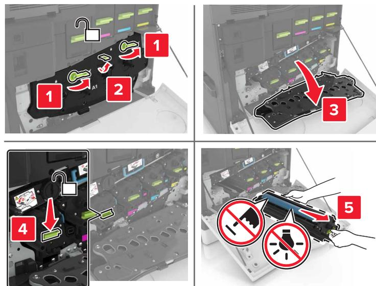
**4** Remove the photoconductor unit.
