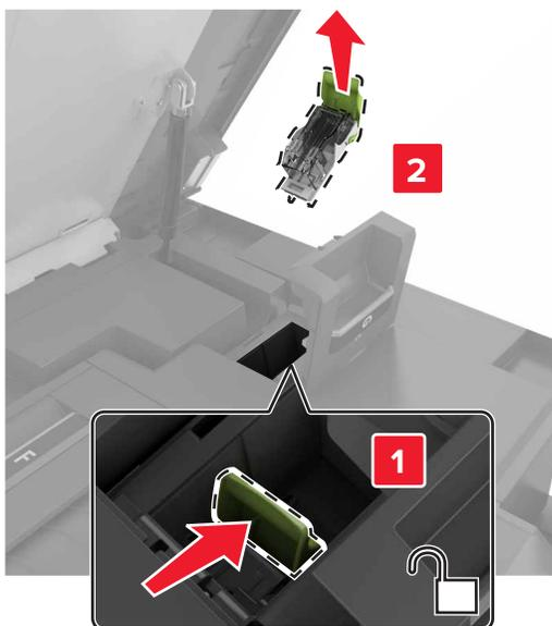
4 Lift the staple guard, and then remove the loose staples.
