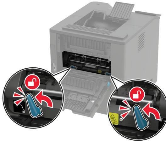
**4** Remove the used hot roll fuser.
