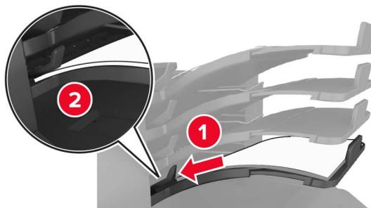
**Note:** If the paper is not under the bin arm, then a jam occurs due to an overfilled bin.
