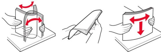
**4** Load the paper stack with the printable side facedown, and then make sure that the side guides fit snugly against the paper.
