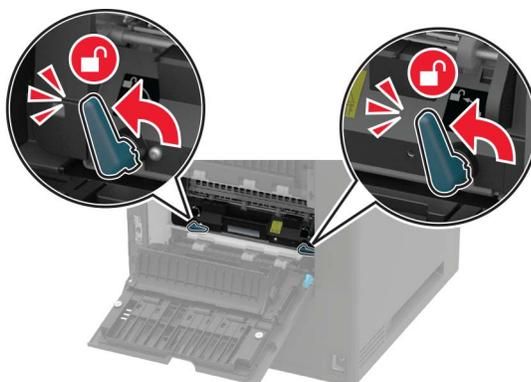
**3** Remove the used fuser.
