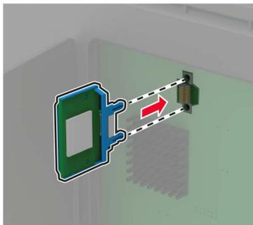
**Note:** The entire length of the connector on the card must touch and be flush against the controller board.
