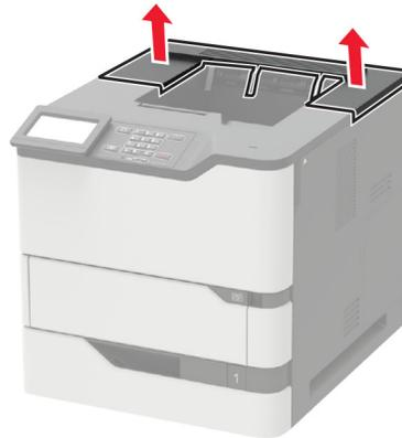
**6** Install the mailbox on the printer., and then push it down to make sure that it is securely attached to the printer.
