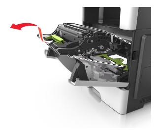
**Warning—Potential Damage:** Do not expose the imaging unit to direct light for more than 10 minutes. Extended exposure to light may cause print quality problems.
