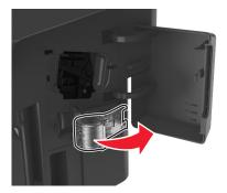
**5** Insert the spare staple case into the staple cartridge.
