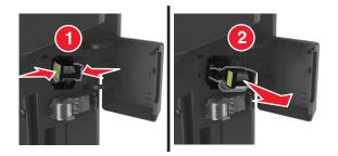
**3** Lift the staple guard, and then remove the loose staples.
