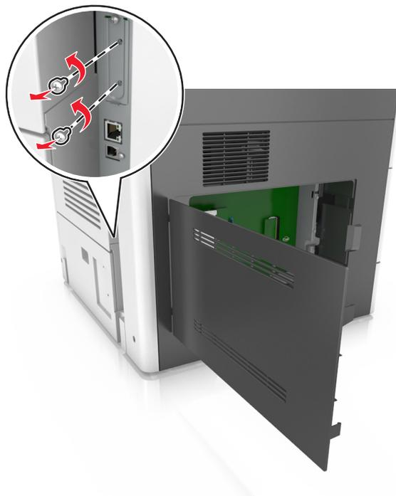
**4** Remove the printer hard disk.
