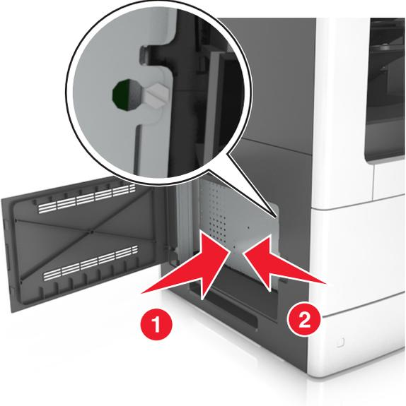
6 Tighten the screws on the shield.
