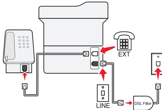
Digital subscriber line (DSL) splits your regular telephone line into two channels: voice and Internet. Telephone and fax signals travel through the voice channel, and internet signals pass through the other channel.
