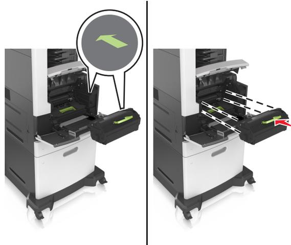
**Warning—Potential Damage:** When replacing a toner cartridge, do not leave the imaging unit exposed to direct light for an extended period of time. Extended exposure to light may cause print quality problems.
