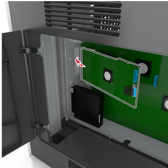
**Note:** Hold the ISP at an angle over the plastic bracket so that any overhanging connectors will pass through the ISP opening in the cage.
