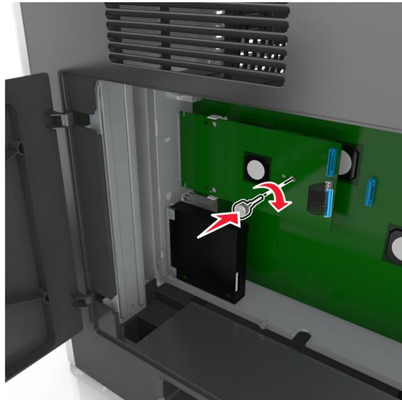
**Note:** Turn the screw clockwise, enough to hold the ISP in place, but do not tighten it yet.
