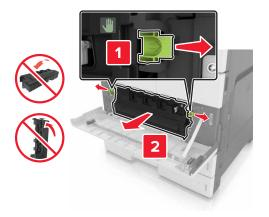
**3** Unlock the photoconductor unit.
