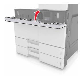
7 Clean the charger and the printhead lens. For more information, see <u>"Cleaning the charger and the printhead lens"</u> on page 205.
