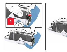
Insert the new cartridge into the cartridge holder.
