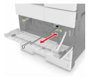
Remove the printhead wiper.
