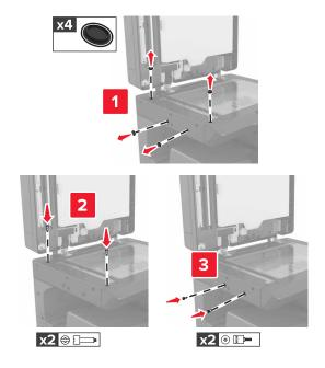
**Note:** Remove the screws after setting up the printer in another location.
