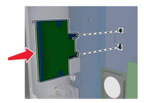
**Warning—Potential Damage:** Improper installation of the card may cause damage to the card and the controller board.
