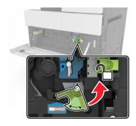
**4** Remove the photoconductor unit.
