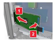
**c** Use the provided thumbscrew for the ISP to attach the ISP to the bracket.
