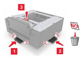
Remove the connector cover from the printer.
