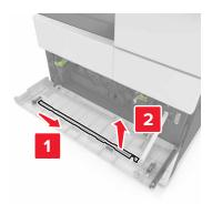
Insert the wiper into the hole until it stops, and then slide it out. Repeat three times.
