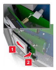
**8** Insert the plug of the hard disk interface cable into the connector on the ISP, and then connect the ISP solution interface cable into the receptacle of the controller board.
