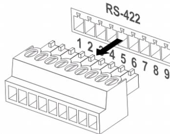
2. Peel off a section of copper wire (AWG Nos. 28 to 18) and insert it into the connector hole; then use flat screw driver to fix it
