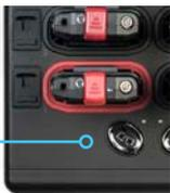
Place the Leader into the red Docking Station pocket. Place Participant and Sub-leader units into the black Docking Station pockets (see diagrams on Page 15). Momentarily press the Pairing Button on the Docking Station. Pairing Indicator will flash during pairing, then turn solid momentarily and finally extinguish when the pairing process is completed. To pair more than 15 Participants and Sub-leaders, repeat the process using the same Leader.
