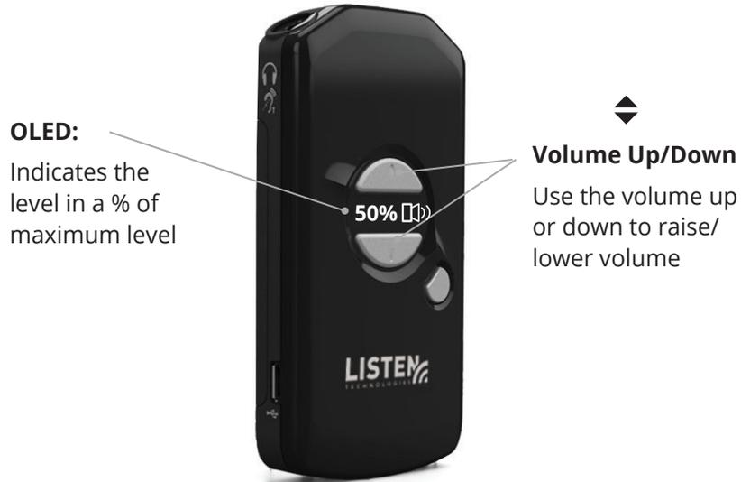
If the volume is adjusted while there is no audio present the unit will output a momentary tone each time the button is pressed allowing the user to gauge and adjust the audio level to a comfortable listening level. The volume level will be displayed for 3 seconds and then the display will turn off.
