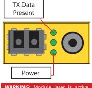
WARNING: Module laser is active as soon as power is connected, regardless of LED indication
