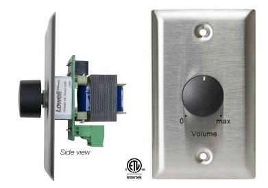
100W ATTENUATOR WITH PRIORITY RELAY (EMERGENCY BYPASS) provides precise level adjustment of single or multiple speaker lines. This unit includes a standard one-gang stainless steel wall plate with black rotary knob.
