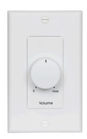
THE LINEAR TAPER POTENTIOMETER VOLUME CONTROL allows an amplifier's control voltage to be set or adjusted from a single remote location. This unit includes a one-gang decorator-style wall plate with rotary knob.
