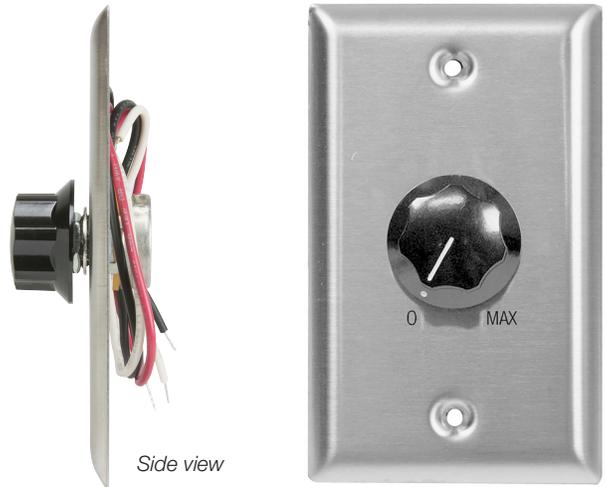
POTENTIOMETER VOLUME CONTROL with 5k ohm impedance provides economical volume level adjustment in systems with low power circuits. This unit includes a standard one-gang stainless steel wall plate with black rotary knob.
