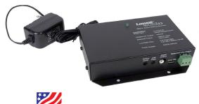
Compact generator produces an analog pink noise signal for systems that utilize a separate amplifier to drive sound masking speakers in order to produce random low-level background noise to mask ambient noise and aid conversational privacy.
