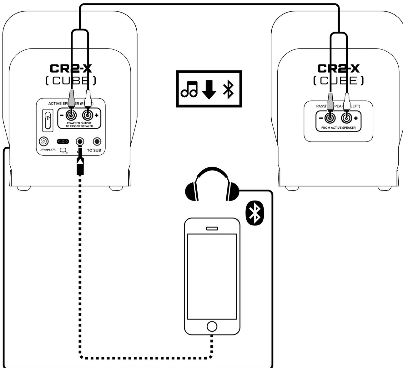
This is a typical use for CR2-X CUBE. This would be a prime example of utilizing it to play music. First, make sure the CR2-X CUBE is positioned for your setup. Next, connect RCA cables from the active speaker to the passive speaker.
