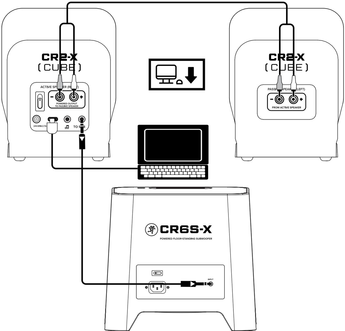
The illustration above shows another typical use for CR2-X CUBE. This would be a prime example of utilizing it for gaming. First, make sure the CR2-X CUBE is positioned for your setup. Next, connect RCA cables from the active speaker to the passive speaker.
