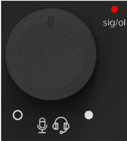
This knob is used to adjust the channel 1 volume – microphone and headset – to the headphones and mix minus.
