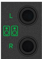
These 1/4" balanced stereo output jacks connect to the input of powered monitors. The signal at this output is a stereo mix of all inputs. This includes channel 1 unless the direct monitor switch is disengaged. The output level is controlled via the monitor output level knob, located on the front of MainStream. [It's the small one located on the right-hand side of MainStream; for reference, the silkscreen printed underneath the knob displays a set of monitors.].
