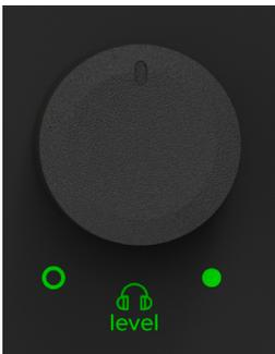
This knob is used to adjust the volume at the 1/4" headphones and 1/8" headset outputs from ∞ (off) to maximum gain (max). Make sure that this knob is fully off before selecting or adding a new source.
