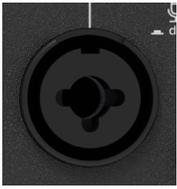
This is a female XLR connector that accepts a mic or line-level input from almost any type of source. Professional ribbon, dynamic, and condenser mics all sound excellent through this input. The mic / line input will handle any kind of level you can toss at them, without overloading.
