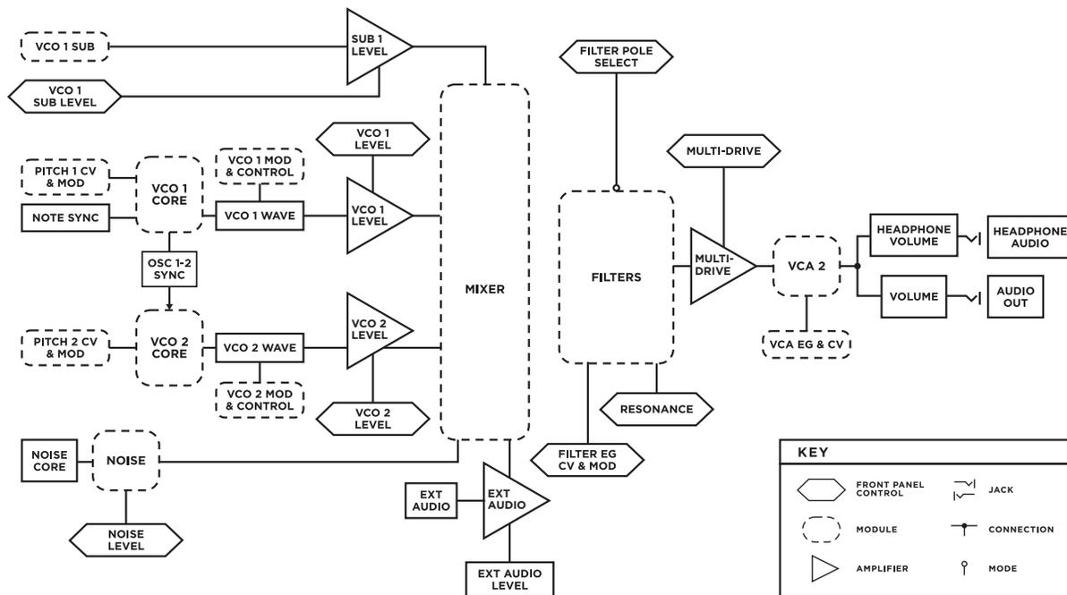
Subsequent 25 can be controlled using control voltages and MIDI commands. When your Subsequent 25 receives either a control signal from the onboard keyboard or a Note On command from an external MIDI source, it responds by sending a gate signal to trigger the envelopes and a control voltage (CV) to control oscillator pitch. The envelopes respond by sending control signals to the amplifier and filter.
