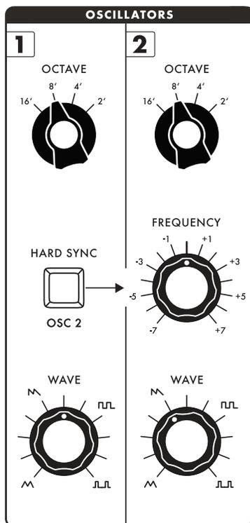
Oscillator 1 and Oscillator 2 are the primary Subsequent 25 sound sources. Each Oscillator generates four basic waveforms: triangle, sawtooth, square, and pulse.
