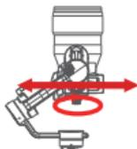
c. Loosen the knob of the roll arm, adjust roll arm leftwards and rightwards until it remains horizontal, and then lock the knob.
