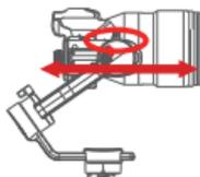
b. Rotate the camera to make its lens face upward, loosen knob on the release plate, adjust the release plate back and forth until the lens faces straight upward, and then lock the knob.
