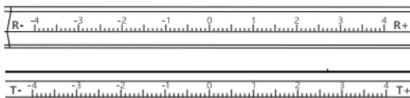
**!** Note: Balance check can be only used with the tilt and roll axis, the pan axis balance can't be checked. When exit balance check, a notice that user need to check and balance pan axis manually will appear on the screen. Be sure that the motor lock has been released when using balance check.
