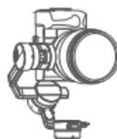
**!** Note: The camera can only be installed vertically using the Arca-Swiss quick release plate. It does not block the camera's battery port and memory card slot.
