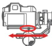
d. Hold the gimbal horizontally to make the pan arm level with the ground, then loosen the knob on the pan arm, adjust the pan arm leftwards and rightwards until it remains level, and then lock the knob.
