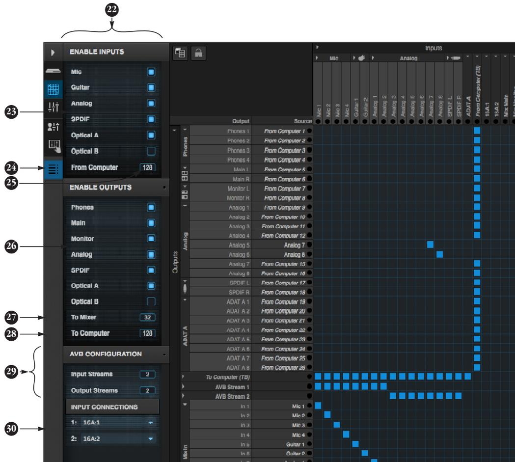
22. Use the Routing Setup sidebar to show and hide inputs and outputs in the routing grid. You can also configure the number of audio channels to/from the computer and network.
