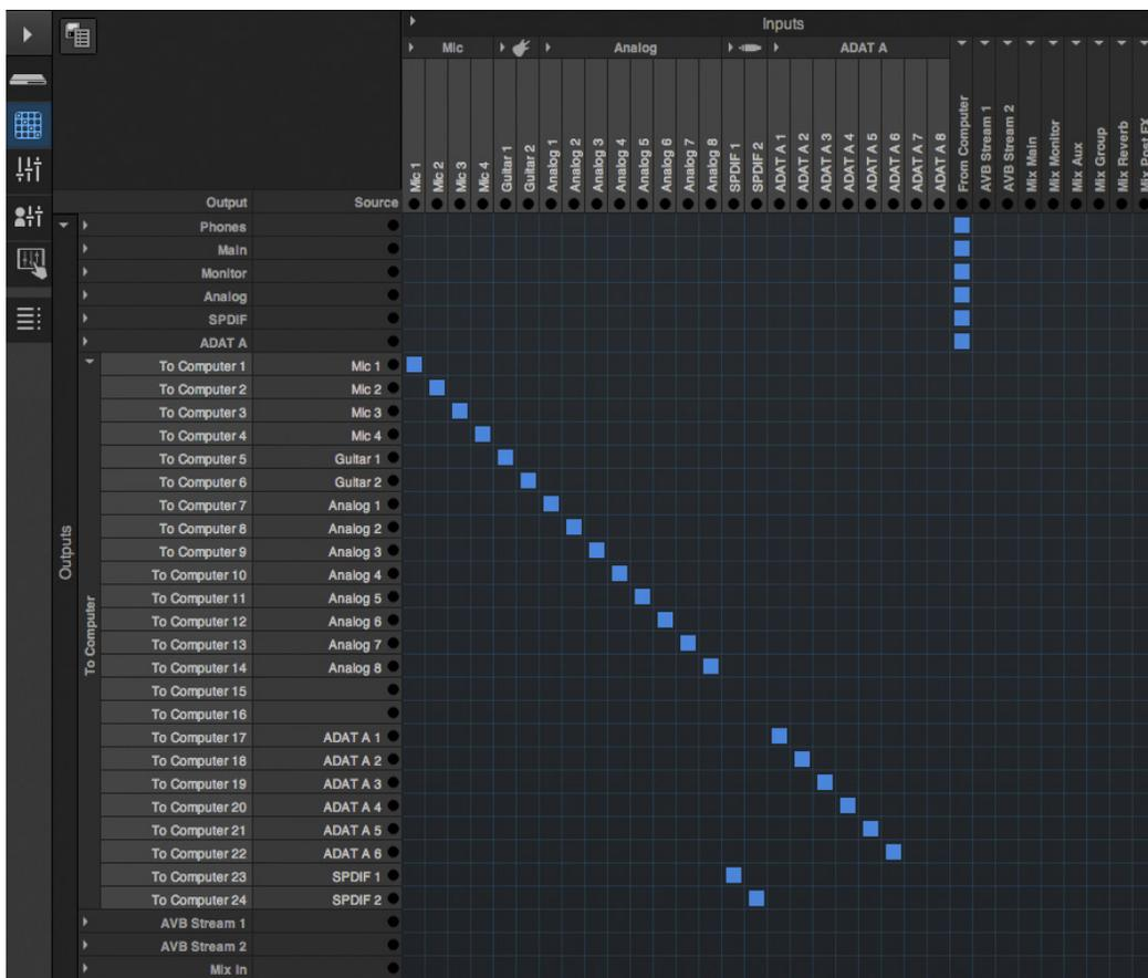
Figure 7-7: An example of routing physical inputs on the 1248 to computer channels (for host audio software). In this example, S/PDIF input is on channels 23-24 going to the computer, and 24 channels total are being used for streaming to the host computer, but more can be added for other inputs from the mixer or AVB network, if any.
