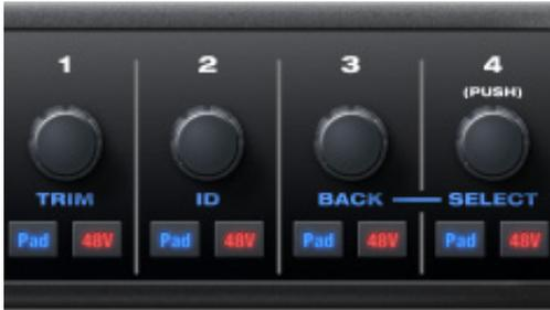
Figure 6-2: Push the knob to activate the functions labeled in blue.
