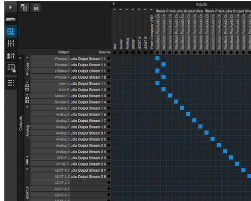
Figure 4-10: Routing Mac channels to physical outputs.
