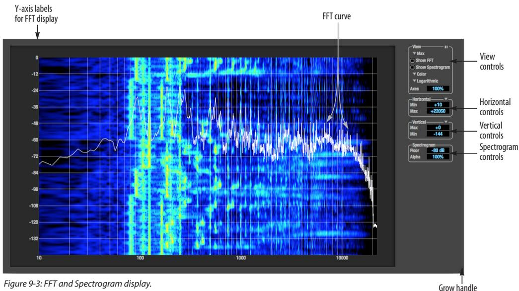
Figure 9-3: FFT and Spectrogram display.
