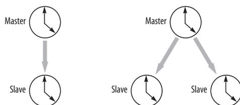
Figure 4-19: To keep your MOTU interface phase-locked with other digital audio devices connected to it, choose a clock master.
