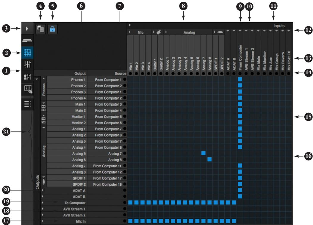
The Routing Tab lets you route inputs to outputs. Outputs are listed by row on the left; inputs are listed in columns across the top. Simply click in the grid to make a single connection. Click and drag to make multiple connections in one gesture. To route a single input to multiple outputs, make multiple connections vertically in the same column below the input. To mix multiple inputs to the same output, you'll need to use the mixer (page 22) and the *Mix In* bank in the routing tab (17).
