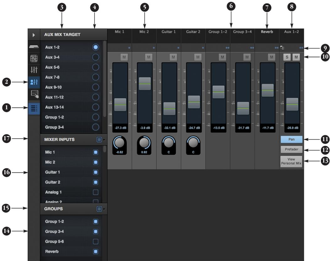
The Aux Mixing tab provides quick access to your MOTU AVB interface's mix busses (aux busses, groups and reverb bus), viewed one at a time. Choose a bus in the Aux Mix Target section and then use the faders to directly mix the send levels from all mixer inputs, groups, and the reverb bus.
