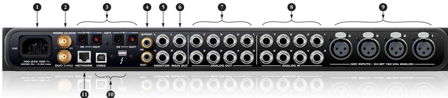
1. The 1248 is equipped with an auto-switching international power supply.
