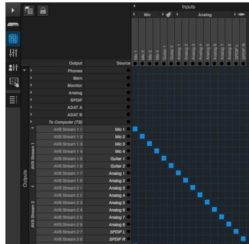
Figure 4-11: Routing physical inputs to the Mac.
