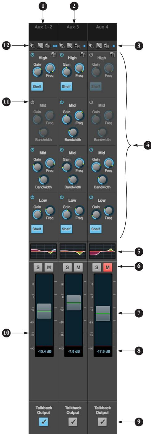
Aux busses can be used to create sub-mixes. An aux bus can be assigned to any output in the Routing grid (page 20).
