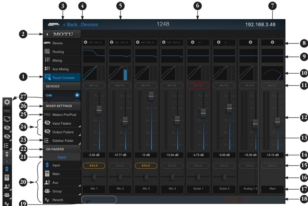
The Touch Console provides touch-screen friendly access to the mixer. It is ideal for mixing on mobile devices like tablets and smartphones. It supports multi-touch operation. For example, you can move multiple faders at the same time with two or more fingers.
