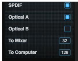
Figure 9-2: The *To computer* setting (item 19 on page 20) determines how many channels you see in the *Left Input* and *Right Input* menus.
