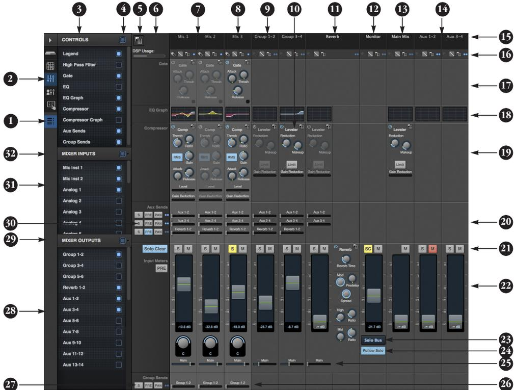
The Mixing tab gives you full access to the 48-channel mixer, which provides a main mix bus, monitor bus, three group busses, seven aux busses, and a dedicated reverb bus. Use the Device tab to configure how many inputs you wish to work with (up to 48). Use the Routing tab (page 20) to route channels to the mixer inputs. Channels can come from any source, such as the physical inputs on the interface or channels from the computer or AVB network.
