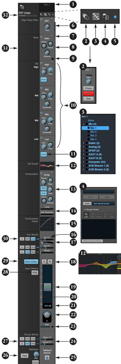
To access a mixer input channel strip, go to the Mixing tab (page 22), reveal the side bar (item #3 on page 22), and show the input channel in the *Mixer Inputs* section (31). To show and hide sections of the channel strip, such as EQ or the compressor, use the *Controls* section of the side bar (item #3 in the Mixing tab on page 22).
