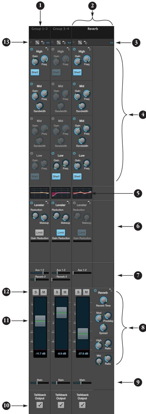
Group busses can be used to create a mix sub-group, which is a set of inputs you wish to control together as a group. Groups differ from aux busses in that they have aux sends, a reverb send, as well as a main mix send. In addition, group busses are equipped with the Leveler.
