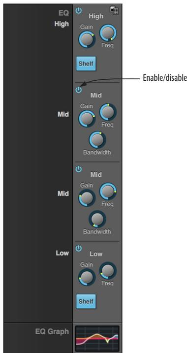
Figure 8-2: The Four-band parametric EQ module.
