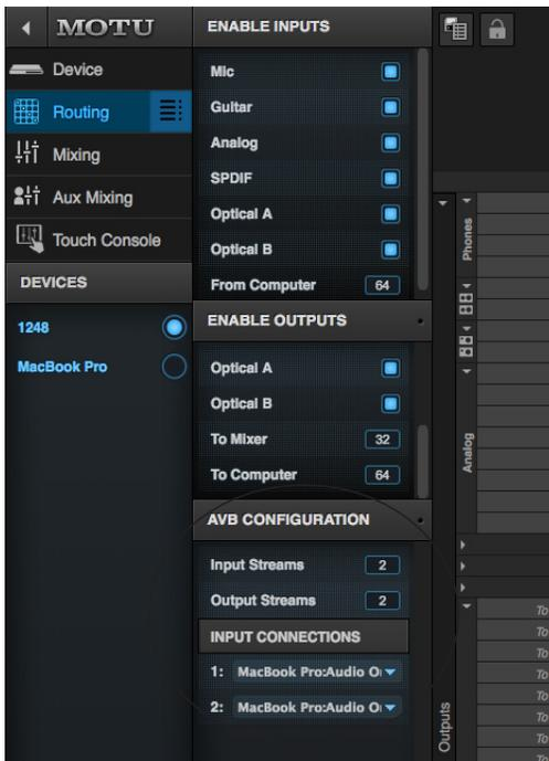
Figure 4-9: Routing computer streams to the interface for playback from the Mac.
