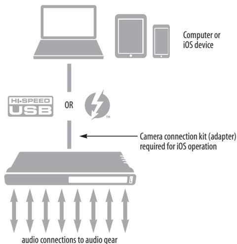
Figure 5-1: Using your MOTU AVB device as an audio interface.
