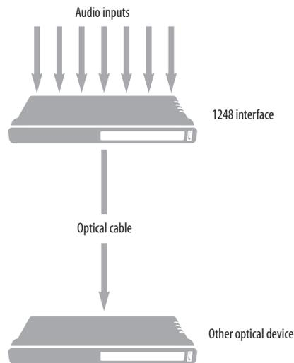
*Figure 5-6: Use the Optical converter preset to connect additional audio inputs and outputs to another optical device. This example shows 1248 interface inputs being routed to the other optical device, but you could also do the same thing for outputs, even simultaneously.*
