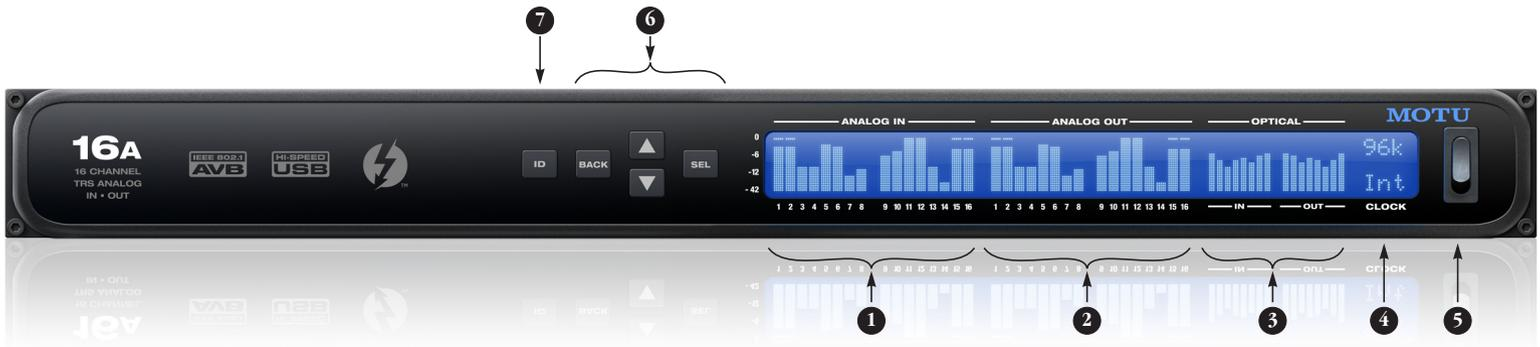
1. ANALOG INPUT METERS for the sixteen balanced (TRS) quarter-inch inputs.
