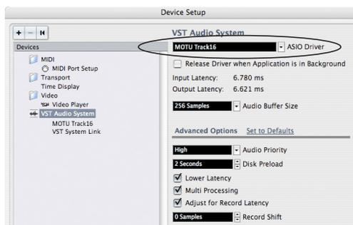
Figure 7-7: Enabling the Track16 in Cubase
