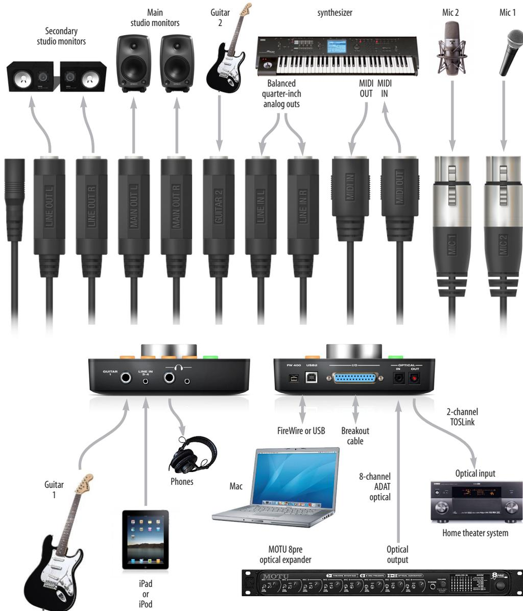
Figure 4-7: A typical Track16 studio setup.
