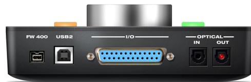
Figure 4-1: the Track16 front and rear panels.
