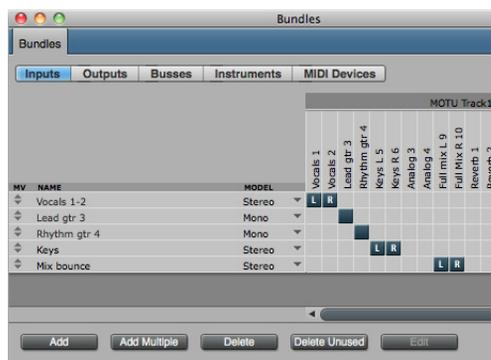
Figure 5-4: Track16 channel names as they appear in Digital Performer.
