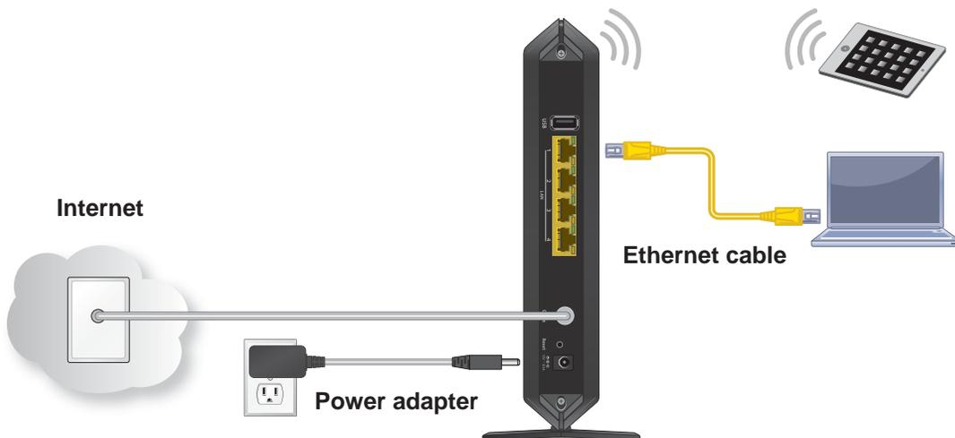
Figure 4. Modem router in a simple network
