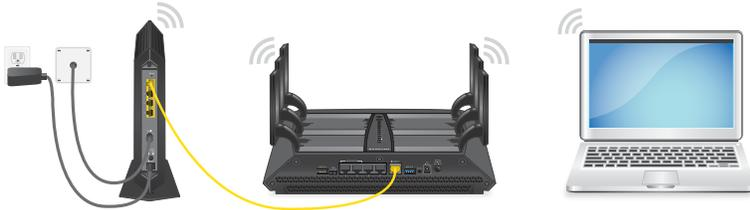
Figure 7. Connect the cable modem to a router
