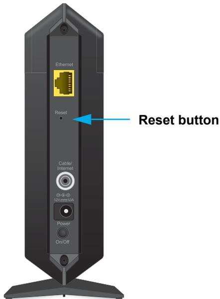
3. Using a straightened paper clip, press and hold the **Reset** button for about seven seconds until all LEDs blink.
