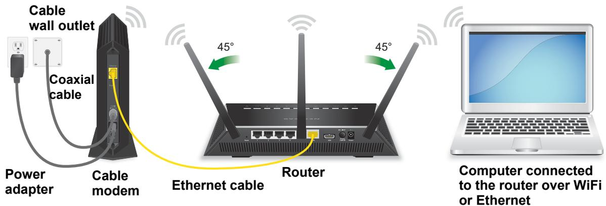
Figure 6. Connect the cable modem to a router
