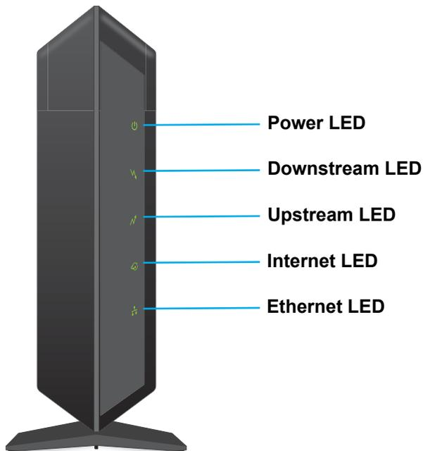
Figure 2. Cable modem front view
