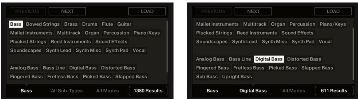
The right display, here when browsing Instruments: Selecting the Bass Type via Knob 5 (left picture) and the Digital Bass Sub-Type via Knob 6 (on the right).
