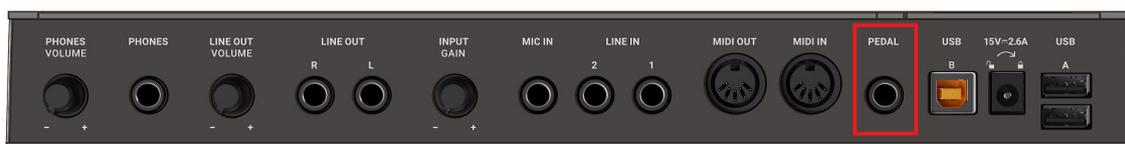
The **PEDAL** socket on the rear panel.
