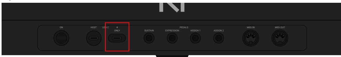
2. Plug the USB-C power supply into the wall outlet.
