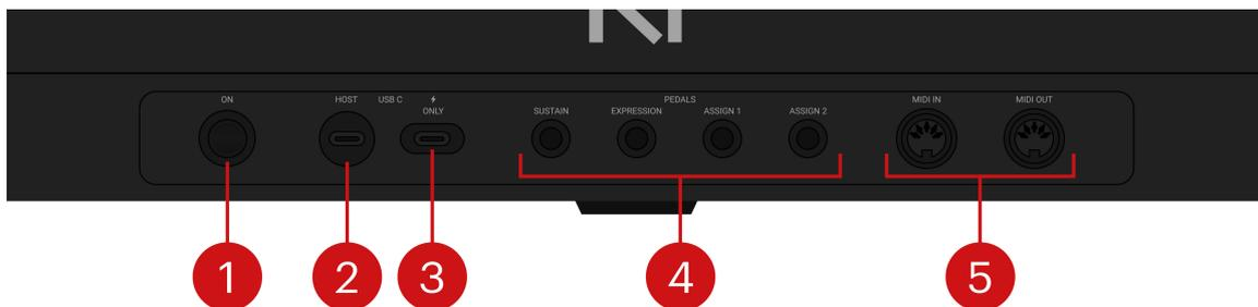
1. **ON switch:** Switches the keyboard on and off.
