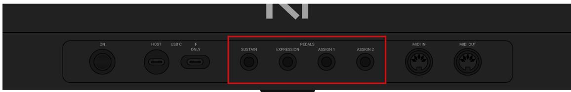
*The pedal inputs on the rear panel of the keyboard.*
