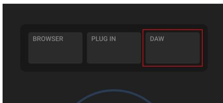
→ The DAW's mixer appears on the display. You can use the display controls, 4-D encoder, and Page buttons to navigate in the mixer and adjust its parameters.
