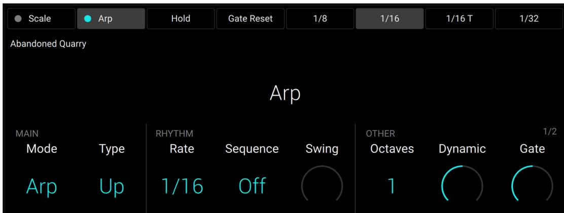
2. Press **SHIFT** + Button 2 (**Arp**) to activate or deactivate the Arpeggiator.
