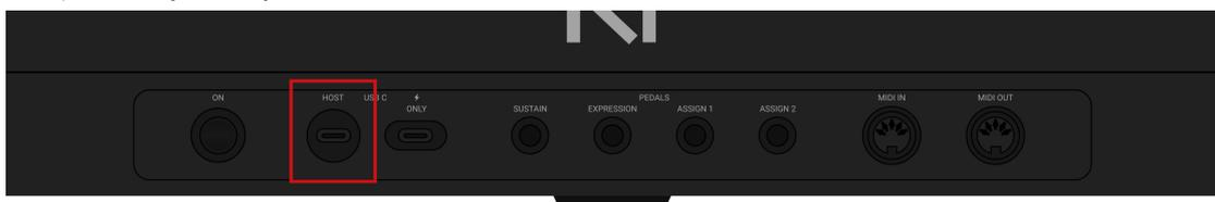
2. Attach the other end of the included USB-C cable to the USB-C to USB-A adapter/cable.
