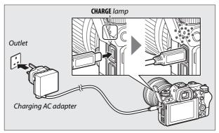
The charging AC adapter can be used to power the camera while the camera is on, but the battery will charge only while the camera is off. The camera **CHARGE** lamp lights amber while charging is in progress and turns off when charging is complete.
