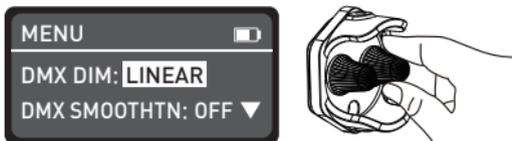
Rotate the "function knob" to DMX DIMMING CURVE.
