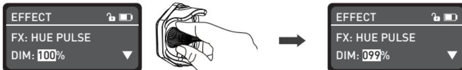
Rotate the "dimmer knob" to set the parameters.
