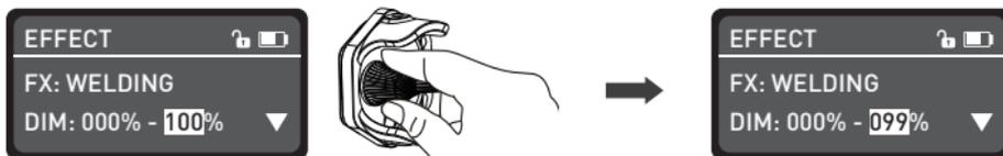
Rotate the "dimmer knob" to set the parameters.
