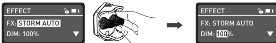
Rotate the "function knob" to select DIM, CCT or INTERVALS.
