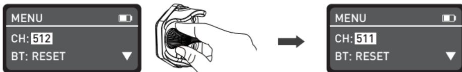
Rotate the "dimmer knob" to set the channel code.
