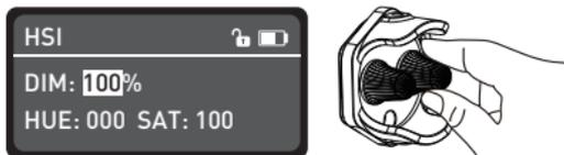
Rotate the "function knob" to select DIM, HUE or SAT.
