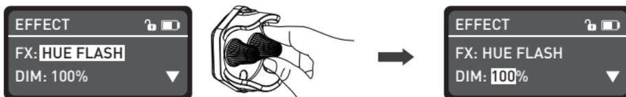
Rotate the "function knob" to select DIM, HUE, SAT or INTERVALS.
