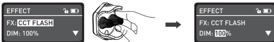
Rotate the "function knob" to select DIM, CCT, G/M or INTERVALS.
