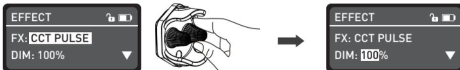
Rotate the "function knob" to select DIM, CCT, G/M or PULSES/MIN.
