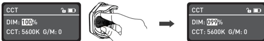
Rotate the "dimmer knob" to set the parameters of DIM, CCT and G/M.
