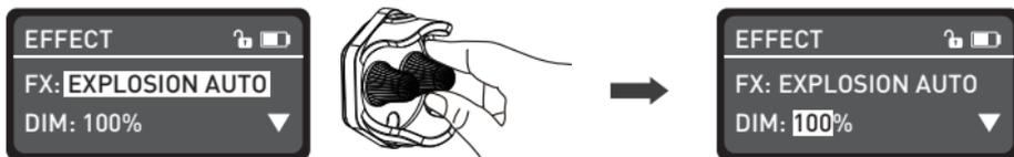
Rotate the "function knob" to select DIM, CCT, G/M, SPEED or DECAY.
