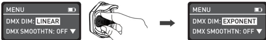
Rotate the "dimmer knob" to select LINEAR, EXPONENT, LOGARITHM, S CURVE or GAMMA 2.2.
