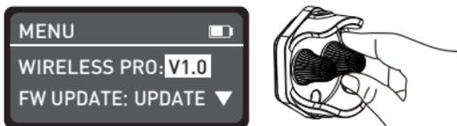
Rotate the "function knob" to WIRELESS PROTOCOL.
