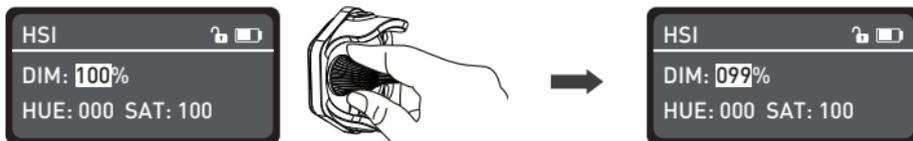
Rotate the "dimmer knob" to set the parameters of DIM, HUE and SAT.
