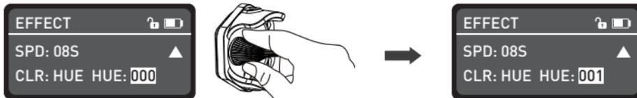
Rotate the "dimmer knob" to set the HUE parameters.
