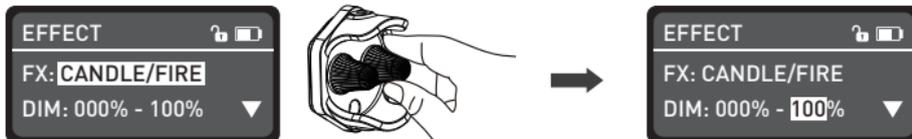
Rotate the "function knob" to select DIM, CCT, G/M or SPEED.
