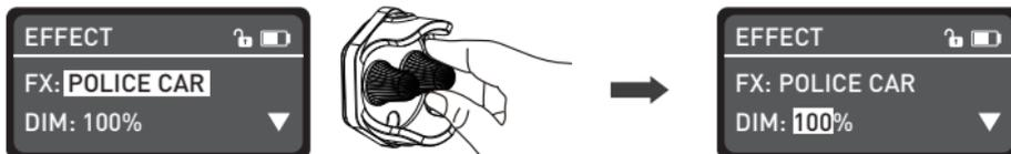
Rotate the "function knob" to select DIM, COLOR or SPEED.
