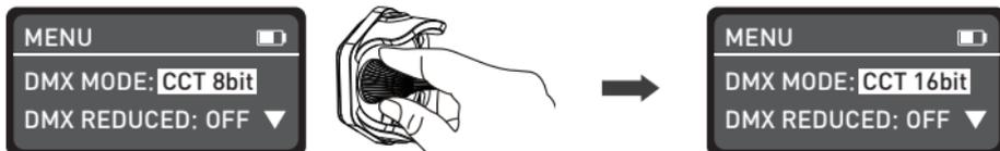
Rotate the "dimmer knob" to select from CCT 8bit, CCT 16bit, HSI 8bit, HSI 16bit, RGBW 8bit, RGBW 16bit, ULTIMATE 8bit, CCT&RGBW 8bit, CCT&RGBW 16bit, CCT&HSI 8bit and CCT&HSI 16bit.
