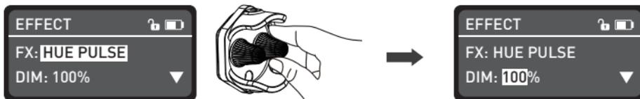
Rotate the "function knob" to select DIM, HUE, SAT or PULSES/MIN.
