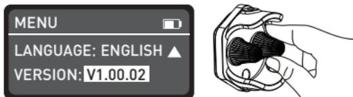
Rotate the "function knob" to VERSION to check the version of the fixture.
