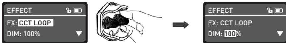
Rotate the "function knob" to select DIM, CCT or SPEED.
