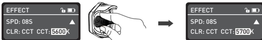
Rotate the "dimmer knob" to set the CCT parameters.
