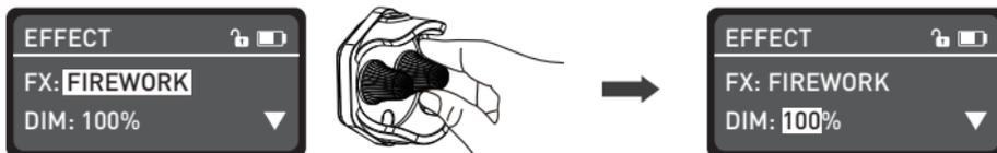
Rotate the "function knob" to select DIM, COLOR, SPEED or DECAY.
