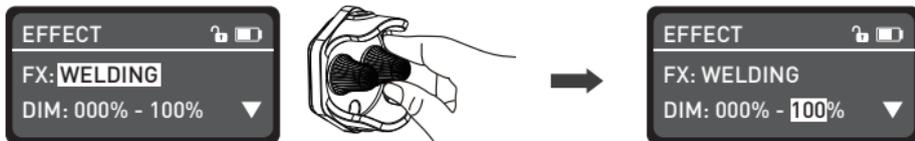
Rotate the "function knob" to select DIM, CCT, G/M, SPEED or PAUSE.
