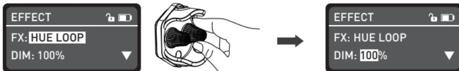
Rotate the "function knob" to select DIM, HUE or SPEED.
