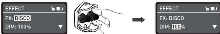
Rotate the "function knob" to select DIM, COLOR or SPEED.
