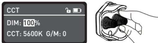
Rotate the "function knob" to select DIM, CCT or G/M.
