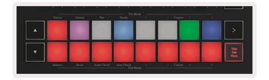
**Solo (Blue)** - Press a pad in the bottom row to solo corresponding tracks, you'll only hear tracks with Solo on. The pads dim if tracks are not soloed (i.e. they are silent). Soloed tracks glow bright blue.
