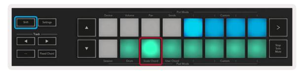
The first and last pad of each row light up more brightly than the middle pads to show root chord position. To navigate between pages of chords use the ▲ ▼ navigation buttons.
