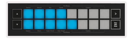
To delete a chord assignment from a pad hold the stop/solo/mute button, the pads with assigned chords will turn red. Press a red pad to delete the assigned chord, once deleted the pad will no longer be lit.
