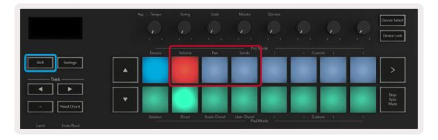
**Volume -** This mode allows you to control Track volumes using the pots. To select this mode, hold the Shift button and press the Volume pad.
