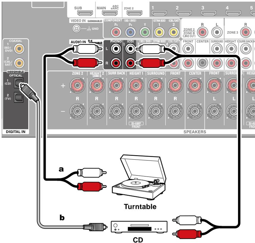
a Analog audio cable, b Digital optical cable
