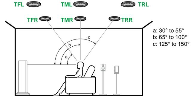
**TFL, TFR** Fit top front speakers on the ceiling in front of the listening position.
