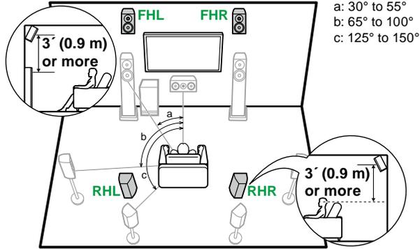
**FHL, FHR** Place the front high speakers directly above the front speakers, angled to face the listening position.
