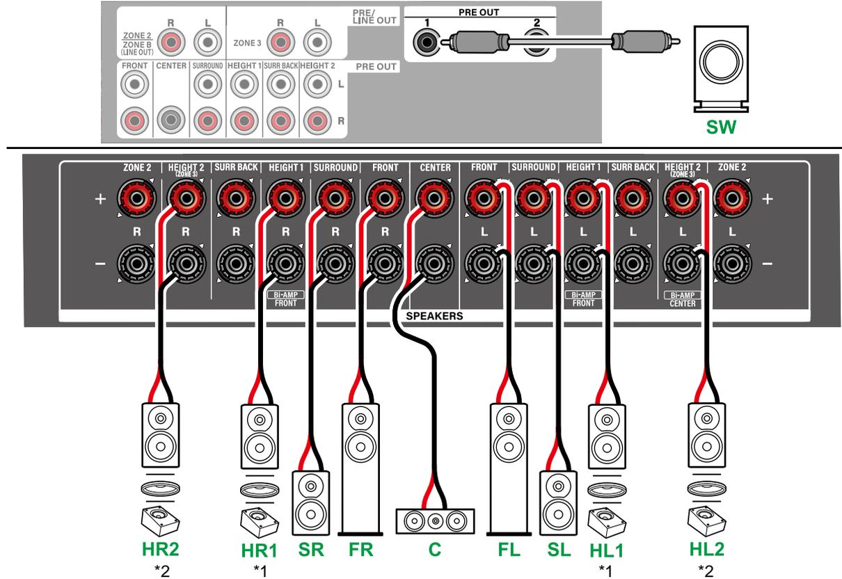
\*1 Connect the Height Speakers you have actually installed (HL1/HR1: Front Height Speakers, Top (front side) Speakers, Dolby Enabled Speakers (Front)).
