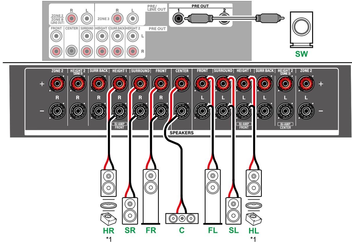
\*1 Connect the Height Speakers you have actually installed (HL/HR: Height Speakers, Top Speakers, Dolby Enabled Speakers).
