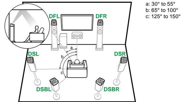
**DFL, DFR** The Dolby enabled speakers (front) are installed on top of the front speakers.
