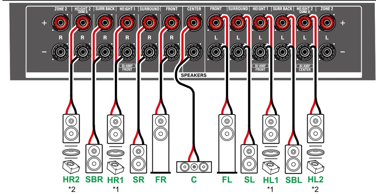
\*1 Connect the Height Speakers you have actually installed (HL1/HR1: Front Height Speakers, Top (front side) Speakers, Dolby Enabled Speakers (Front)).
