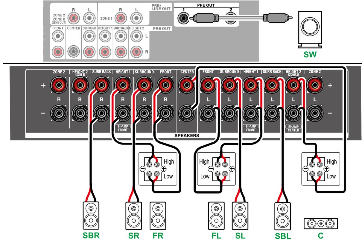
Be sure to remove the jumper bar connecting between the woofer jacks and tweeter jacks of the Bi-Amping supported speakers. Refer to the instruction manual of your speakers as well.
