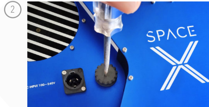
Unscrew the fuse plug connector.
