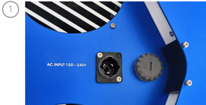
The fuse plug is located next to the AC port.
