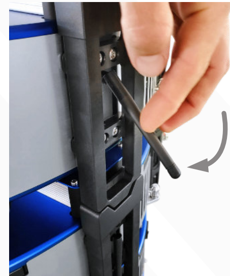
③ Ensure that antennas are stowed away for safe storage.
