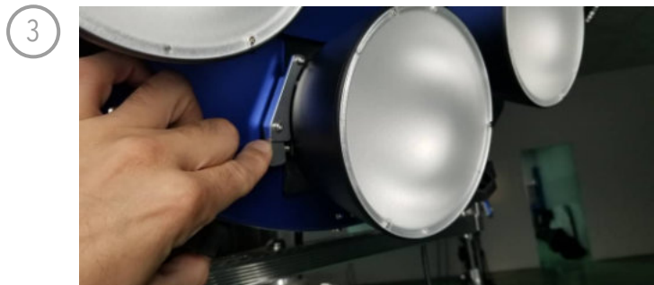
To release the modifier, push the release latch in and twist the lens to the left.
