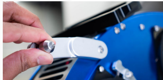
Carefully retract spring loaded pin for attachment.
