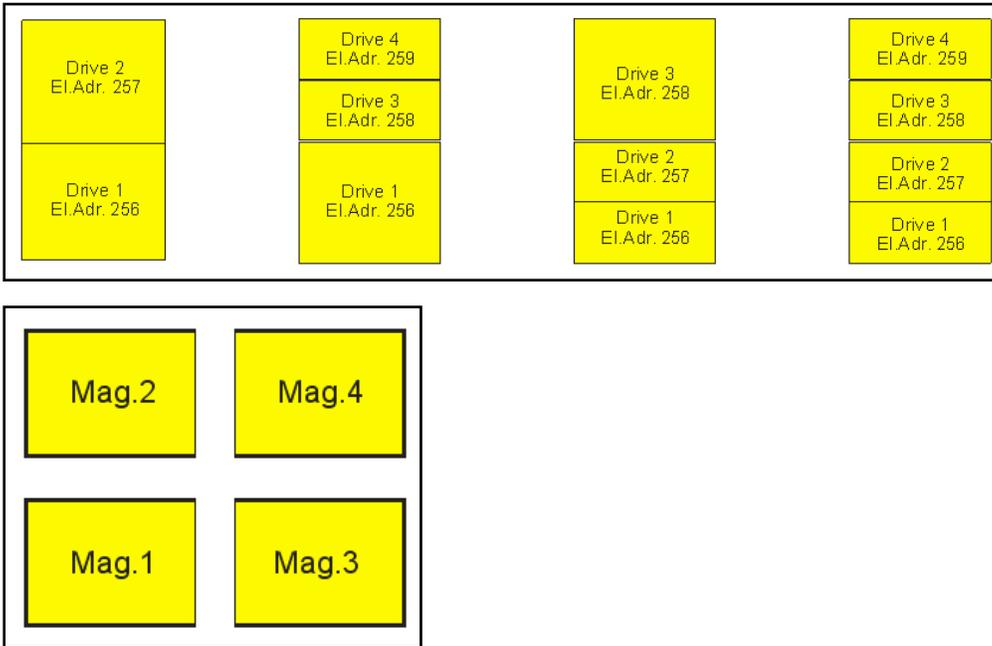
**Figure 69 1-Partition-System (drives and correlated magazines)**
