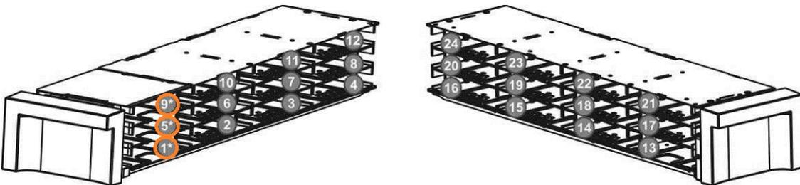
Figure 15 Slot numbering scheme (2U – Triple mail slot)
