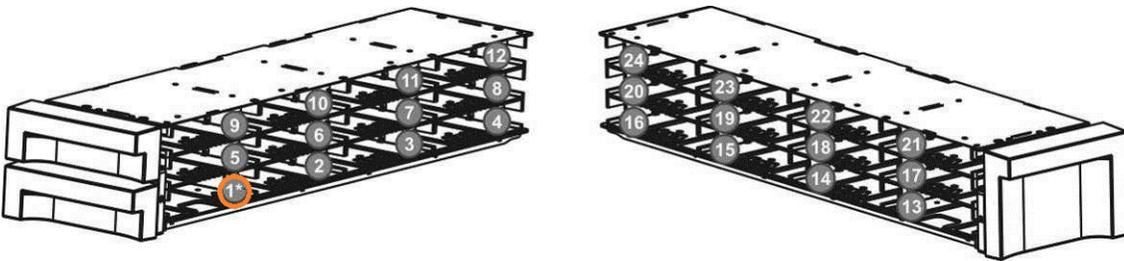
Figure 14 Slot numbering scheme (2U – Single mail slot)
