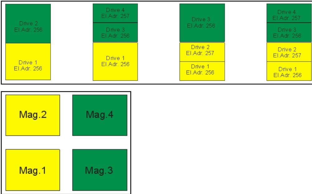
**Figure 70 2-Partition-System (drives and correlated magazines)**
