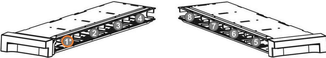
Figure 13 Slot numbering scheme (1U)
