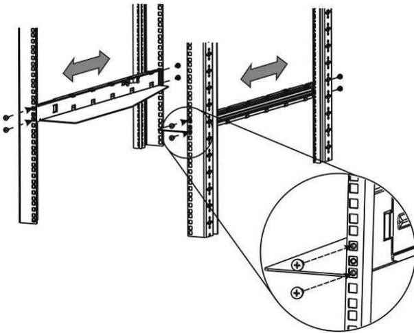
**Figure 4 Install the rack rails (1U)**
