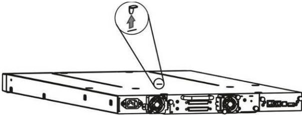
**Figure 2 Remove the shipping lock**
