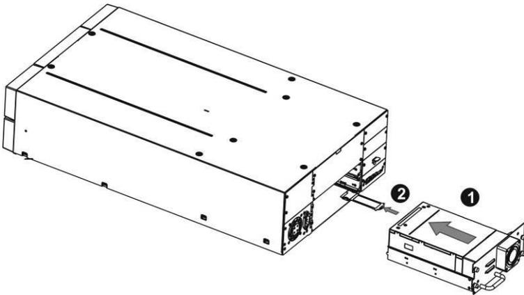
**Figure 8 Install a tape drive (4U)**
