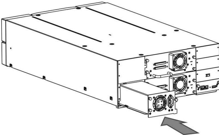
**Figure 10 Install a power supply (4U)**
