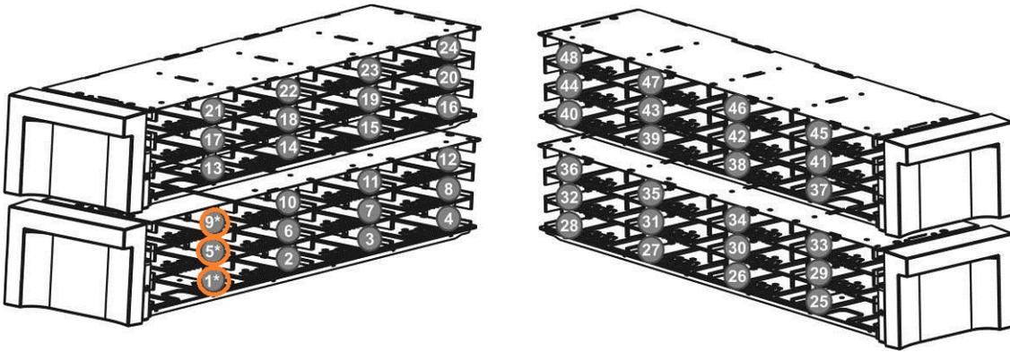
Figure 16 Slot numbering scheme (4U)
