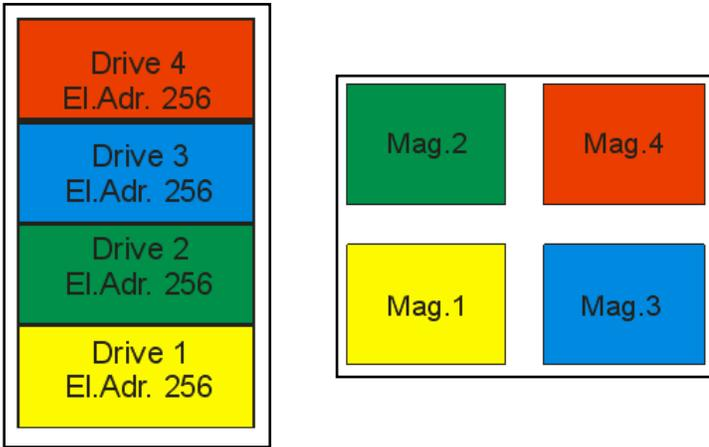
**Figure 72 4-Partition-System (drives and correlated magazines)**
