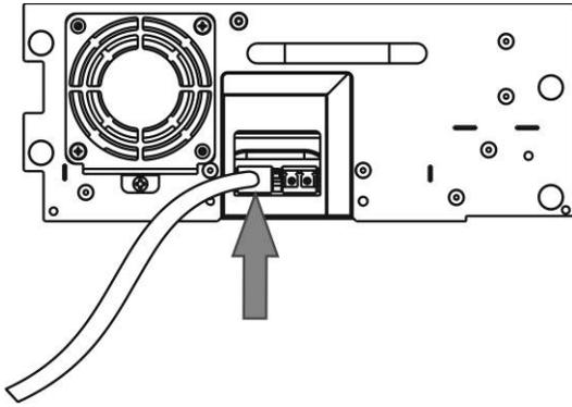
**Figure 11 Connect the FC cable**
