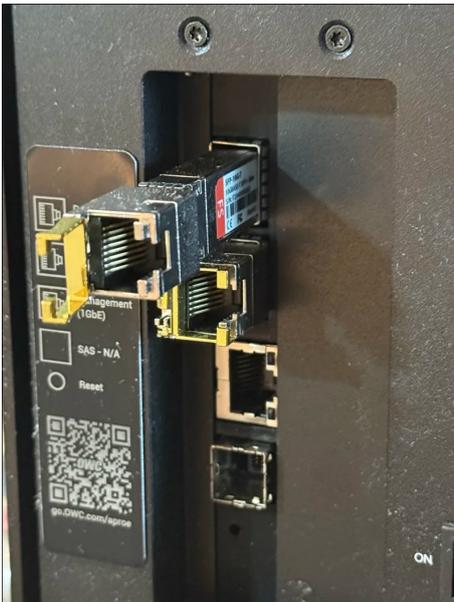
3. Carefully install a desired 10GBase-LR SFP+ | 10GBase-SR SFP+ | SFP+ DAC optic module/cable (not included).
