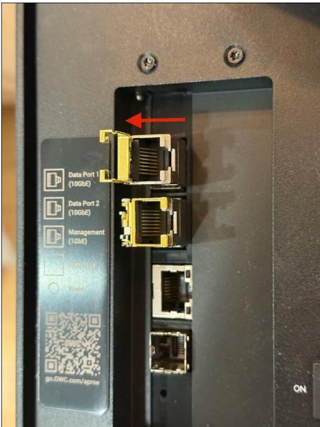
2. Slide the optic module out of the OWC Archive Pro Ethernet.
