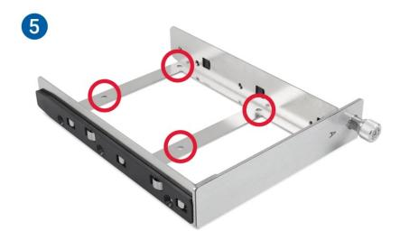
**6.** Place the hard drive inside the drive tray as shown. The label should face up and the SATA connectors should be on the far rear corner of the drive.
