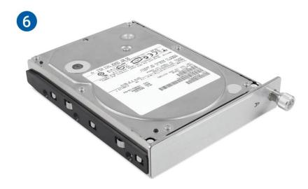
**7.** Fasten the drive into the drive tray using six of the included screws (three per side)
