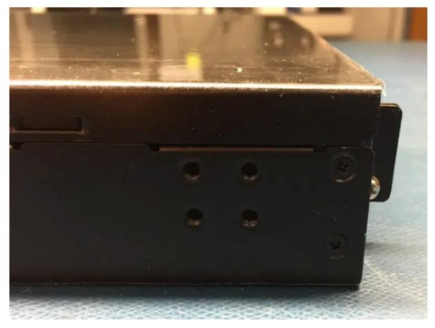
**3.** Affix the rack ears with the rack ear screws to the OWC Flex 1U4 once the desired placement is achieved.
