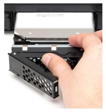
**6.** Press the drive tray door to finish pushing the drive into the drive bay and completing the connection.
