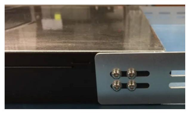
**4.** Carefully place the OWC Flex 1U4 in a rack cabinet. Affix the other end of the rack ears to the rack cabinet.
