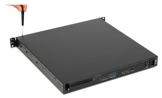
2. Remove the screw holding the PCle slot cover.
