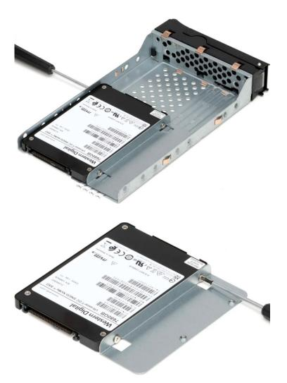
**5.** Insert the drives, with the drive label facing upwards. Carefully push the drive tray forward into the drive bay. Do not force the drive as a minimal amount is needed. The drive will rest slightly protruded outside the drive bay. **NOTE**: The drive trays have locking mechanisms. Ensure the locks are not engaged before installing the drive trays. The lock is disengaged when the locking mechanism is in the up position.
