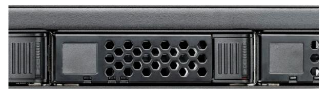
**3.** Disengage the drive tray by pushing the tray tab to the right. The drive tray will protrude slightly from the chassis. Carefully remove the drive tray and place on a flat surface.
