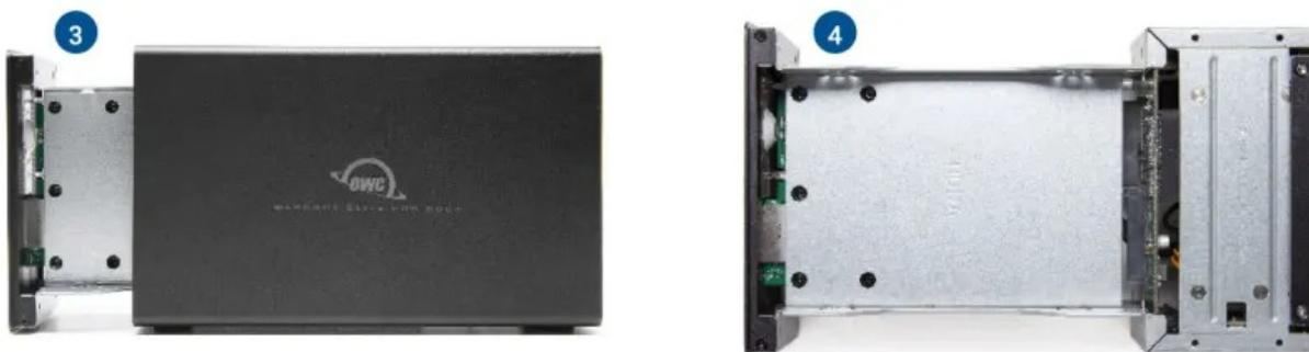
5. Set a 2.5-inch or 3.5-inch SATA drive into the drive housing. The label should be facing upwards. Carefully seat the drive. Minimal force is needed.
