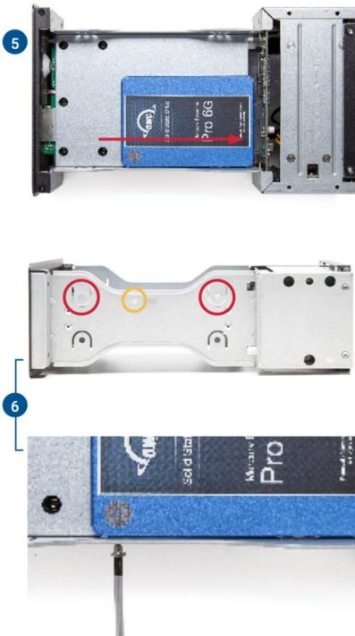
6. Ensure the ports on the back of the inner chassis and the port cut-outs on the back of the outer enclosure are oriented the same way, then slide the inner chassis into the outer enclosure so that the chassis' front plate is flush with the cover's front edge.
