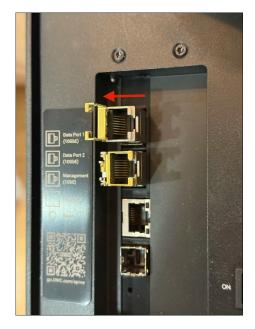
2. Slide the optic module out of the OWC Archive Pro Ethernet.
