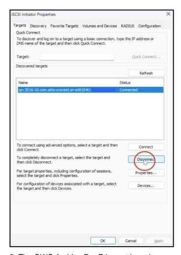
3. The OWC Archive Pro Ethernet is no longer connected to the Windows PC.
