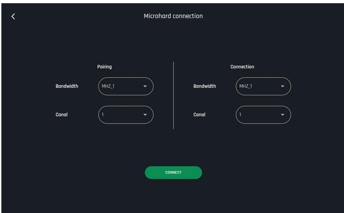
10. **Do not modify** the "Pairing" options (left on the screen) and set the Connection Bandwidth to "MHZ\_4" (4 MHz - right of the screen: refer to the next screenshot).
