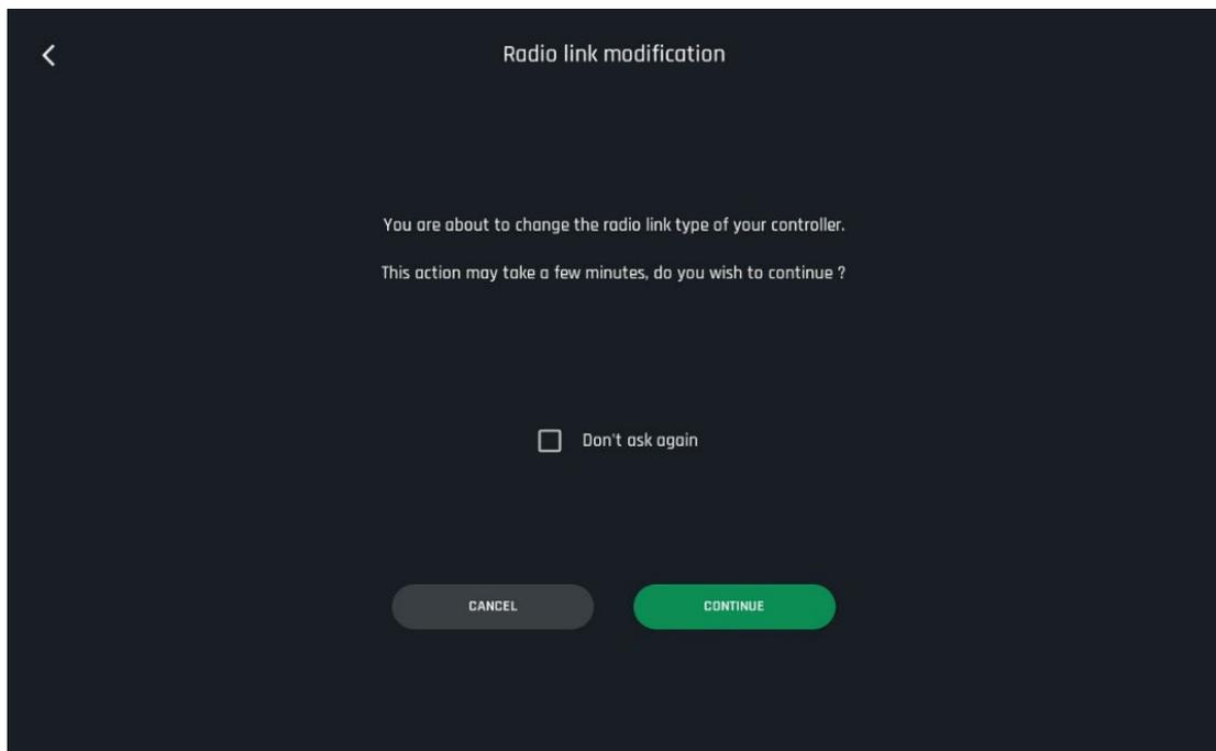
3. Tap the "Don't ask again" box if required, then tap "CONTINUE". The fan of the **Skycontroller USA** Microhard module starts up and the controller displays the following screen.
