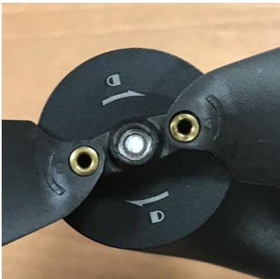
**B. blades:** unscrew damaged B blades (left back & right front) clockwise and screw new ones counterclockwise.
