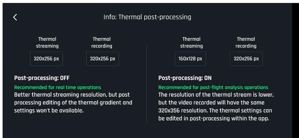
**About Thermal calibration:** **AUTO** mode is recommended for most users. If you select the **MANUAL** mode, note that the application will periodically remind you to calibrate your thermal camera, through the dedicated
