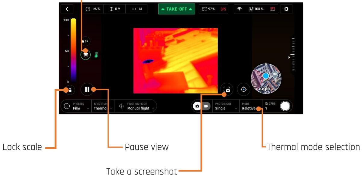
⚠ **Note that when post-processing is activated (default value), the “Pause view” and “Lock scale” buttons are available** – they disappear when post-processing is deactivated (refer to the *“PREFERENCES - Thermal - Thermal post-processing”* section of this guide for further information on thermal post-processing).
