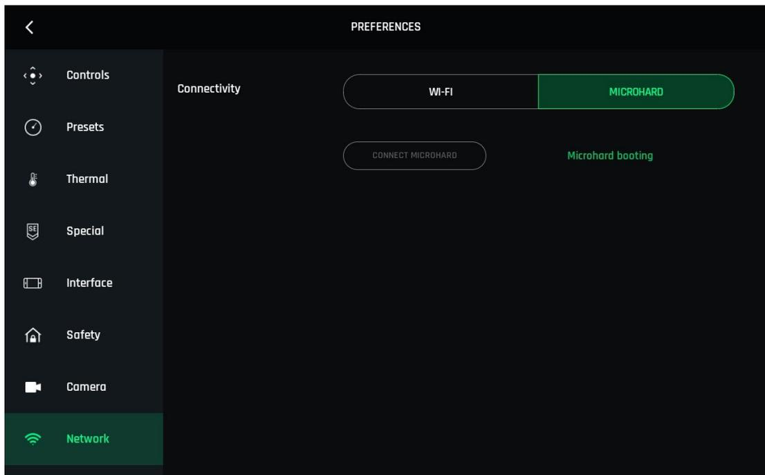
4. Wait about one minute for the Microhard to boot and the "CONNECT MICROHARD" button to activate as on the following screen.
