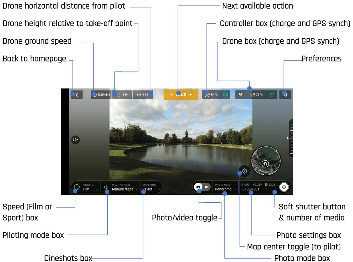
ANAFI USA's photo modes include a Single shot mode, a Burst mode, a Bracketing mode, a Timer mode, a Timelapse mode, a GPS Lapse mode and a five-format Panorama mode.
