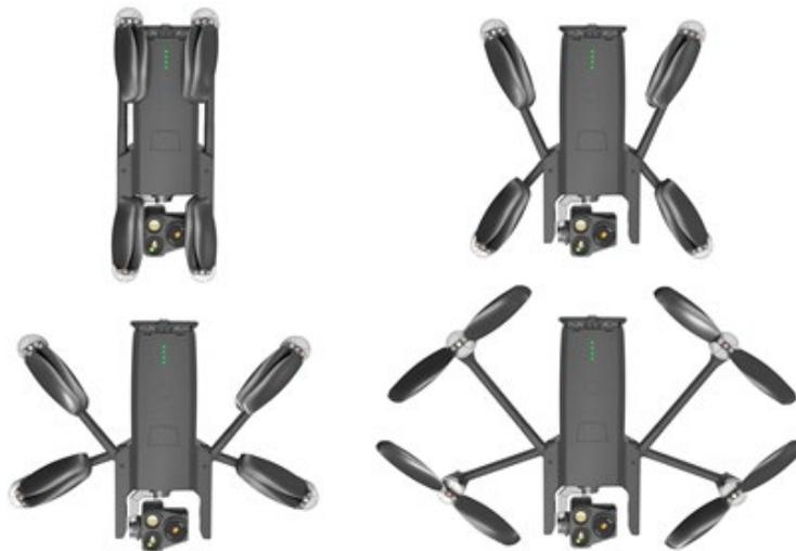
Propeller replacement requires no tool: they just screw in the direction opposite to that of the rotation of motors, without risk of losing small mobile parts.
