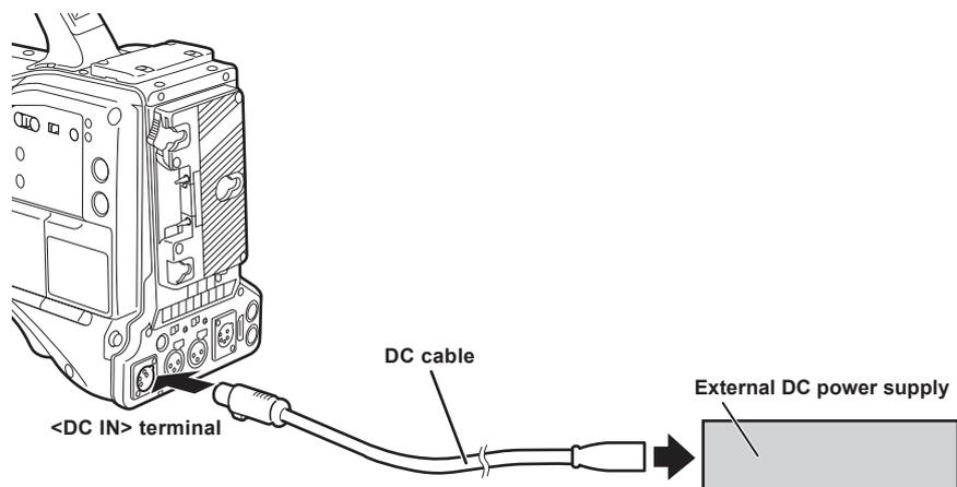
**1** Connect the external DC power supply to the <DC IN> terminal of the camera.
