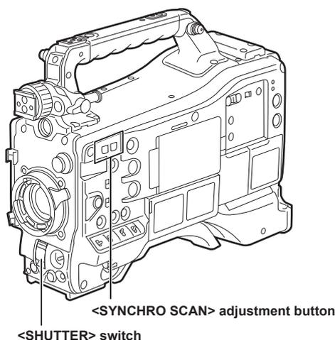
**1** Press the <SHUTTER> switch from the <ON> side towards the <SEL> side to set the camera to synchro scan mode.
