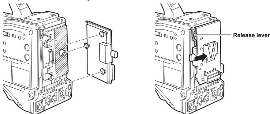
**1** Mount the V-mount type battery plate.
