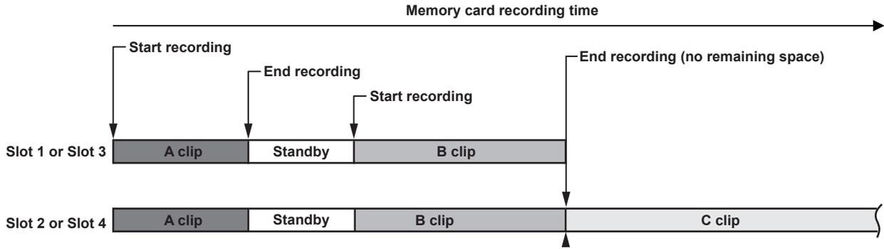
Selecting [ON] in the main menu → [REC/PB] → [REC FUNCTION] → [SIMUL REC] will set the camera to simultaneous recording mode.
