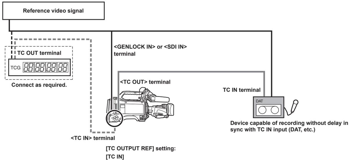
■ When the external device is locked to the time code generator of the camera connected in a cascade configuration
