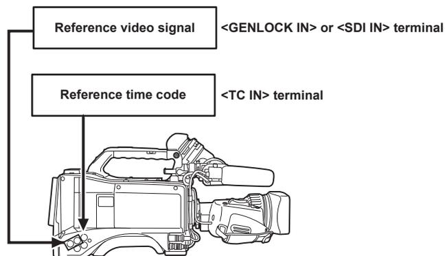
■ When the external device is locked to the time code generator of the camera
