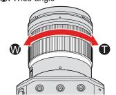
• Rotating the zoom ring displays the focal length on the recording screen.
