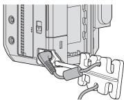
4 Fit the HDMI cable and USB connection cable to the clamp.
