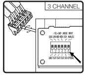
3. For 3 channels connect the speakers to the two outer sets of terminal for your left and right channels and the center set for the center channel. Set dip switch 5 in the down position.
