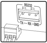
1. Connect the RS232 control device to the RS232 port on the P3-35. Refer to Step 1 of "Speaker Connections" for instructions on wiring the Euro-Block connector.
