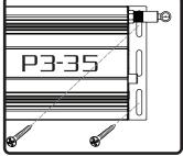
6. If mounting to a flat surface use 2 screws through the mounting bracket on each end of the amp.
