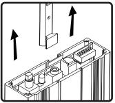
4. Slide mounting bracket into groove on bottom of amplifer enclosure.
