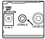
1. Connect the 1/8" mini plug from the IR receiver to the External IR port on the P3-35.
