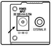
1. Connect the 32v power supply barrel connector to the power input on the P3-35.
