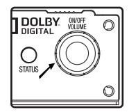
3. Turn the P3-35 on by pressing the on/off button. The LED will turn white when on.
