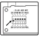
2. To use the internal P3-35 crossover set to 120Hz set dip switch 1 to the up (Sub) position.
