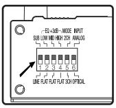
3. To use an external Sub crossover set dip switch 1 to the down (line) position.
