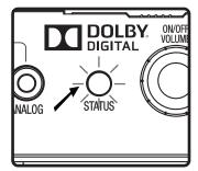
2. Press and hold the mute button on the remote control for 3 seconds then release. The P3-35 LED will blink white for 1 minute or until paired.
