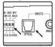
1. For digital connections connect an optical cable from your source to the optical input on the P3-35. Set dip switch 6 in the down position.
