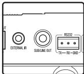
1. Connect a Subwoofer to the P3-35 with an Audio RCA cable.
