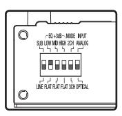
2. To boost the low frequencies set Dip switch 2 to the up position (+3dB)
