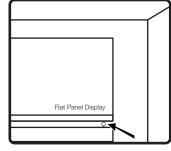
2. Position the IR receiver on a surface that faces out into the area you will be using the remote control. Fasten the IR receiver with the supplied two-sided tape disk.
