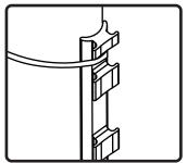
2. Attach mounting bracket to a secure pole or surface using screws or metal strapping.
