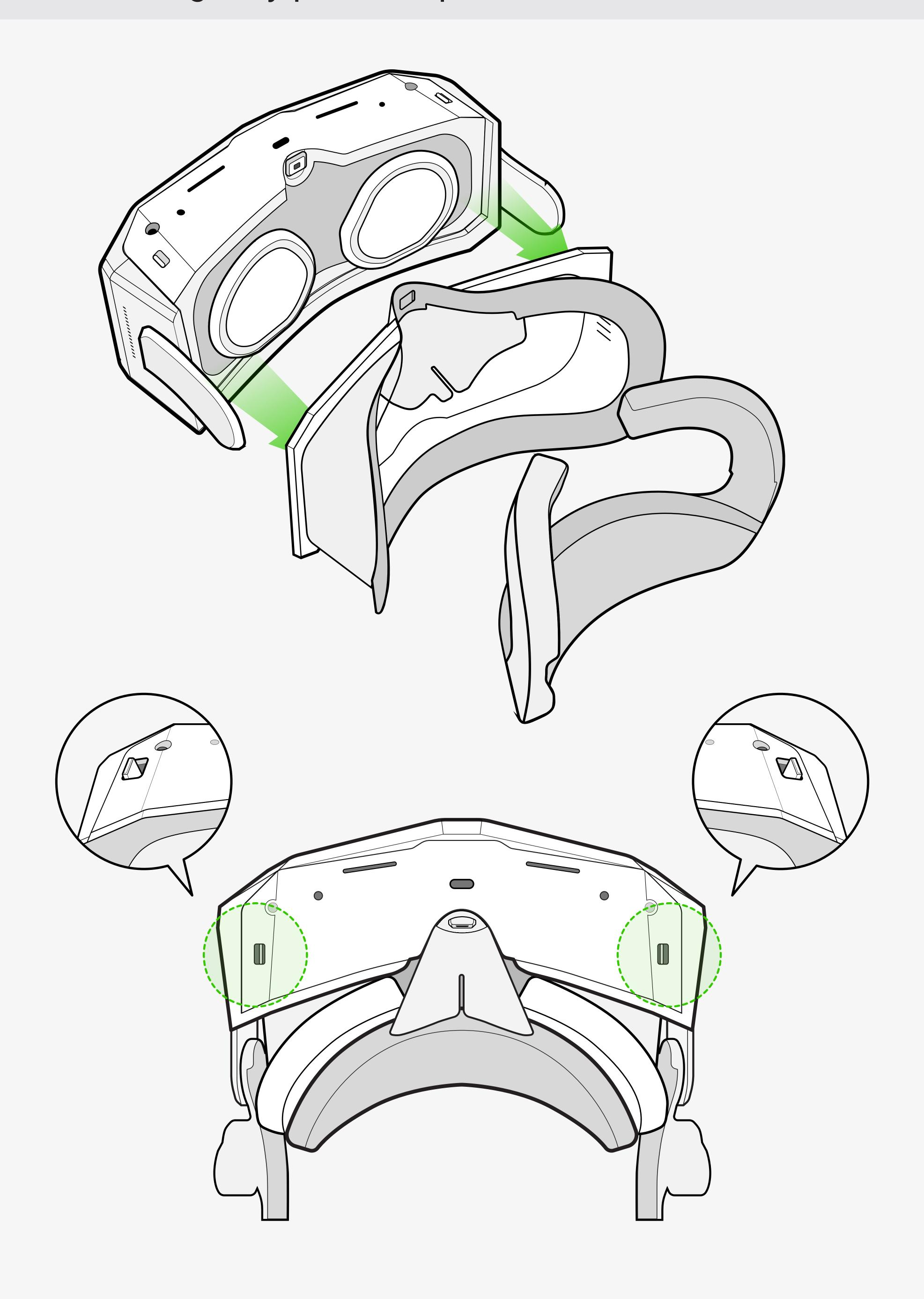
Step 2: Align the optical module and insert it until you hear a "click," ensuring it sits flush with the device body. Reattach the foam and silicone face mask securely.
