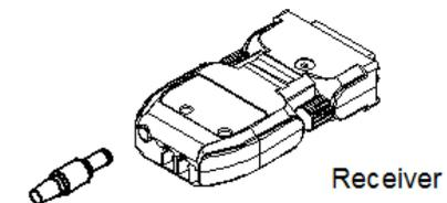
Figure 3 – Connection of power adapter to the receiver
