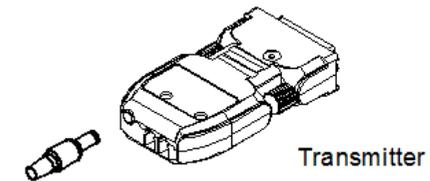
Figure 2 – Connection of power adapter to the transmitter
